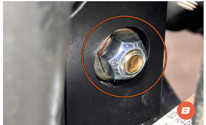
13 A/B. Use one of the supplied \frac{1}{2} "x 5" bolts, two washers, and lock nut to install the shock to the lower auxiliary shock mount. One washer must be installed between the shock and the lower mount as shown. 13 B. Install the second washer at the inside of lower auxiliary bracket then install the lock nut. Torque to 75 ft lbs. Note: For proper lock nut engagement, one to two threads must be exposed past lock nut.
