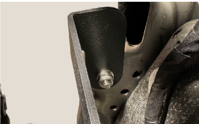
18. Use a 10mm socket/wrench and the supplied M6 flange bolt, M6 washer, and locknut to mount the rear bracket to the left side of seat frame. Hand tighten only.
