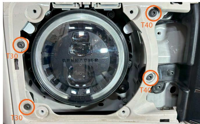
**6.** Use a T30 and a T40 Torx bit to remove the 4 painted headlight panel screws.
