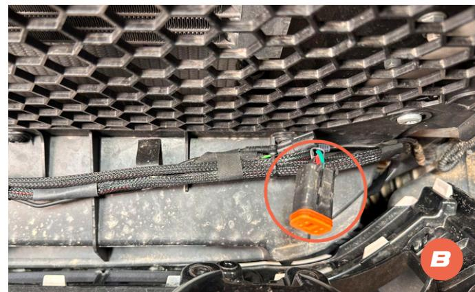
**22 A/B.** Route the supplied light wire harness starting from the right fog lamp opening to the left fog lamp opening.
