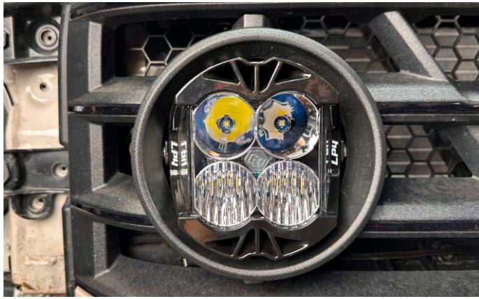
**30.** Re-install the fog lamp bezel rings using the factory hardware.
