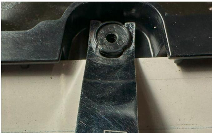
**13.** Remove the remaining clips using a clip removal tool. Remove all 4 retaining clips.
