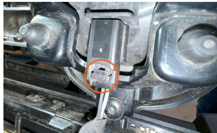
**16.** Push tab and pull on connector to disconnect light.
