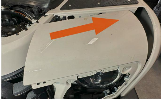
**32.** Come in at an angle when installing the painted headlight panel.
