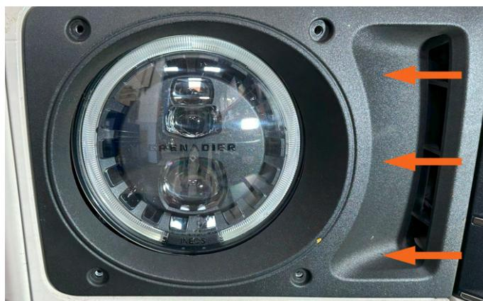
**5.** With the four bezel screws removed, pull out bezel starting from the headlight side and then pull out at angle to unclip bezel from grille.
