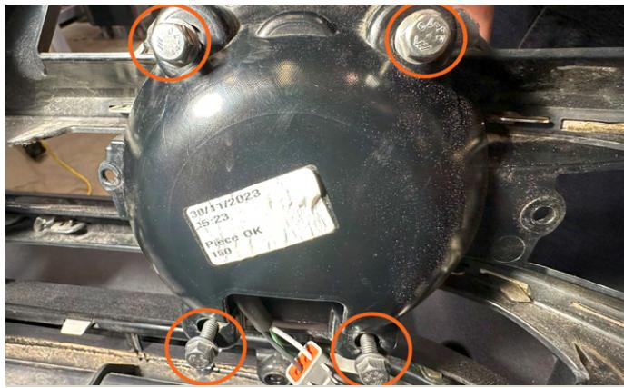
**29.** Use the supplied M6 flange bolts to install the light assembly.
