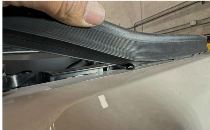
**37.** Start the weatherstrip installation from one end and work around until all t-clips are re-attached. Slide weatherstrip onto one end of t-clip then stretch weatherstrip and let it snap back until the clip is completely inserted in weatherstrip.
