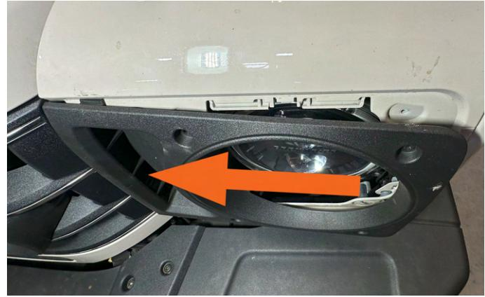
**36.** Come in at an angle when installing the headlight bezel then snap bezel into place.
