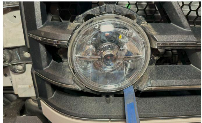
**18.** Use a plastic pry tool and starting from the bottom of the fog lamp pry the lamp straight forward.
