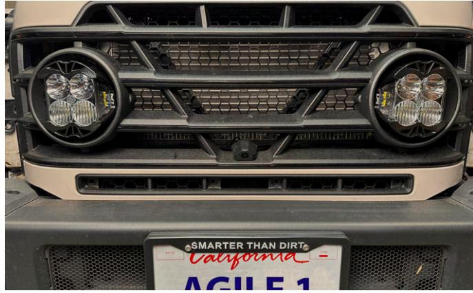
**31.** With both bezels installed, re-install the 4 lower grille bolts from step 13. Re-assemble grille and headlight panels using factory hardware. Refer back to steps 1-13.
