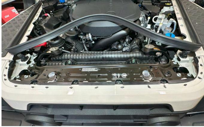
**3.** Unclip the weatherstrip from the upper grille panel only. To avoid damaging the t-clips, do not remove the t-clips from the grille panel.
