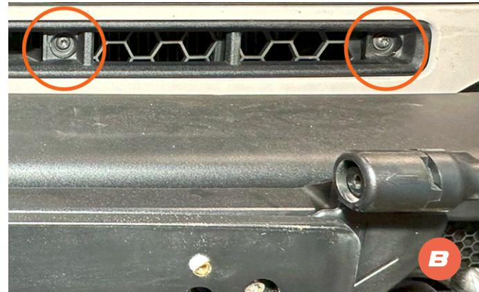
**14 A/B.** Use a T30 torx bit to remove the 4 lower grille bolts. Removing these lower bolts will allow the grille to be tilted forward to ease in the removal of the OEM lights and the installation of the new Agile Light Kit.
