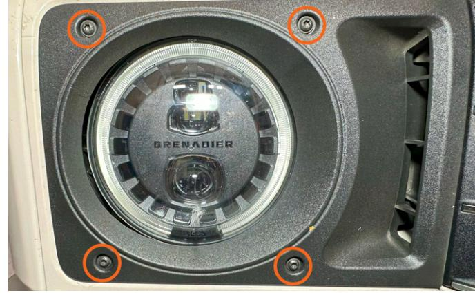
**4.** Use a T30 torx bit to remove the 4 headlight bezel screws.
