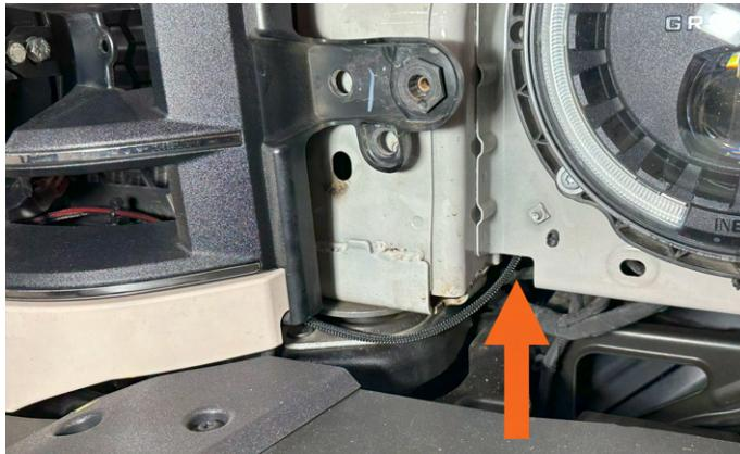
**23.** Continue routing the light wire harness under the headlight assembly to the engine compartment as shown.
