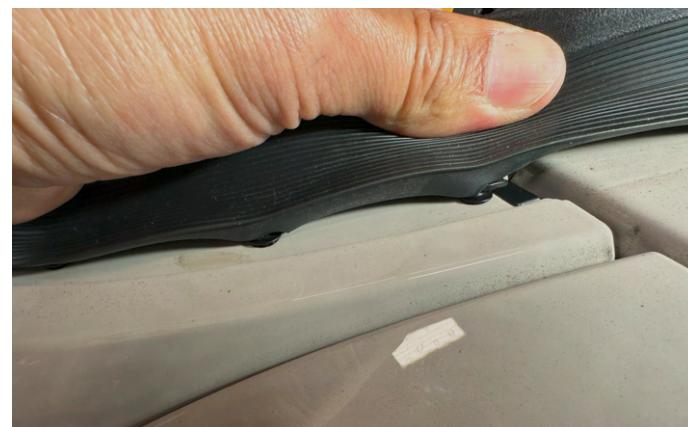
**2.** The hood weatherstrip is attached to the body panels using retainer t-clips. Carefully slide the weatherstrip off retainer t-clips by pulling forward, out and then back on the weatherstrip at each t-clip location.
