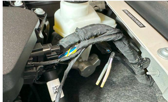
**24.** Locate the light purple wire and the black wire pair. This pair of wires are taped to the large wire harness. Remove tape.
