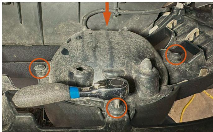
**17.** Use a T25 torx bit to remove the four fog lamp bezel ring screws.
