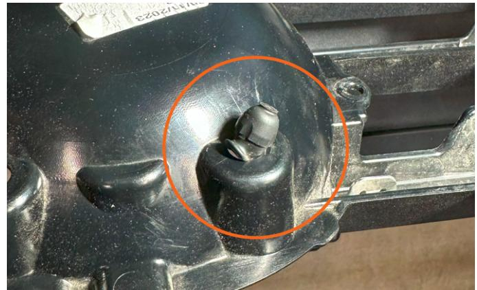
**20.** Remove the 3 grommets from the back side of the grille.
