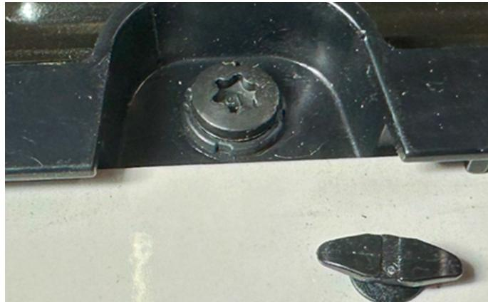
**12.** Use a T30 Torx bit to remove the retainer clip center screw.
