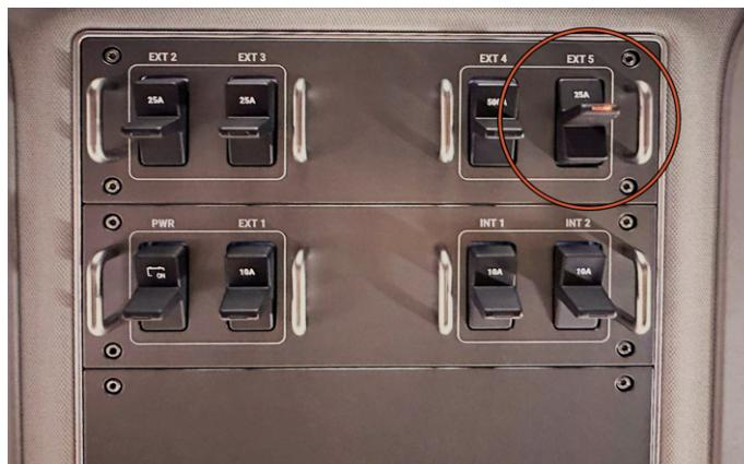
**25.** Turn on the ignition without the engine running. Turn on EXT 5 switch on the Overhead Panel.
