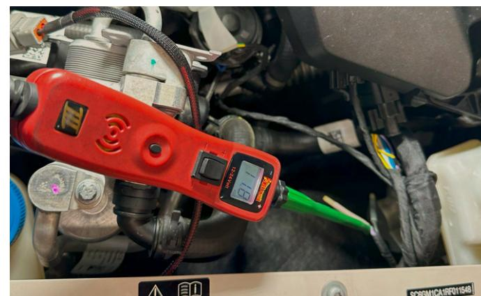
**26.** Test the purple wire for power. Turn off switch and ignition. Splice both purple and black wires and use the supplied butt connectors to join to the light wire harness.
