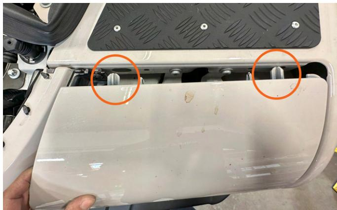
**33.** Now line up panel pins with the holes in fender. When lined up, push panel into place.
