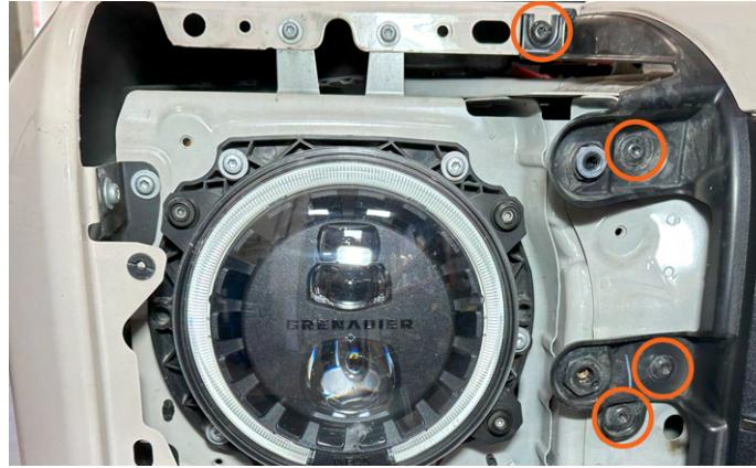
**10.** Use a T40 Torx bit to remove the 4-side grille retaining bolts. Repeat steps 4-10 on opposite side.
