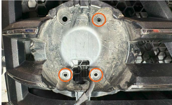
**19.** With the OEM fog lamp removed locate the 3 rubber grommets.
