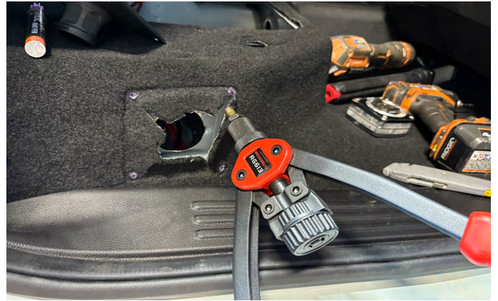
16. Install the supplied M6 nut inserts using the supplied installation tool or tool of choice.
