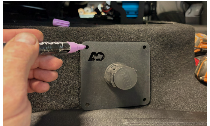
14. Use the Air Couple Plate Assembly as a template to mark the four mounting holes.
