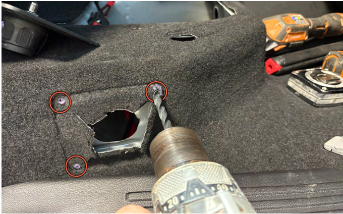
15. Use a 25/64" drill bit at the four marked locations.
