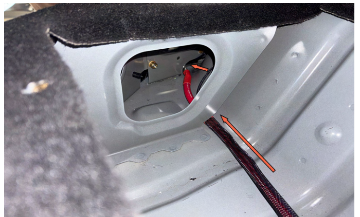
18. Route the battery cable harness from the storage panel cavity to the rear passenger door sill.
