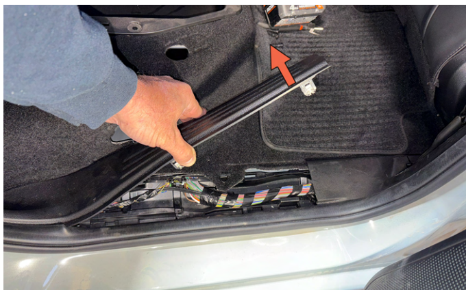
17. Pull up the door sill panel starting from the front until the bottom is completely detached.
