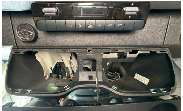
16. Carefully set the cup holder tray in front of center panel.
