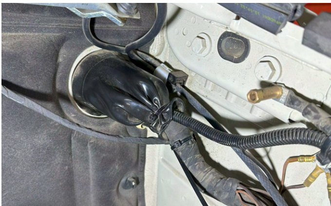
17. At the engine compartment, remove the zip tie from the driver side dust boot. Remove the insulation foam from the inside of dust boot.
