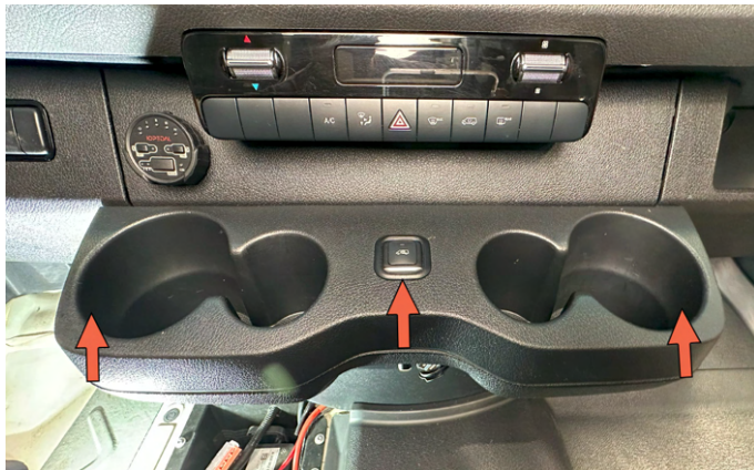
15. Remove the center cup holder tray by pulling up on tray.
