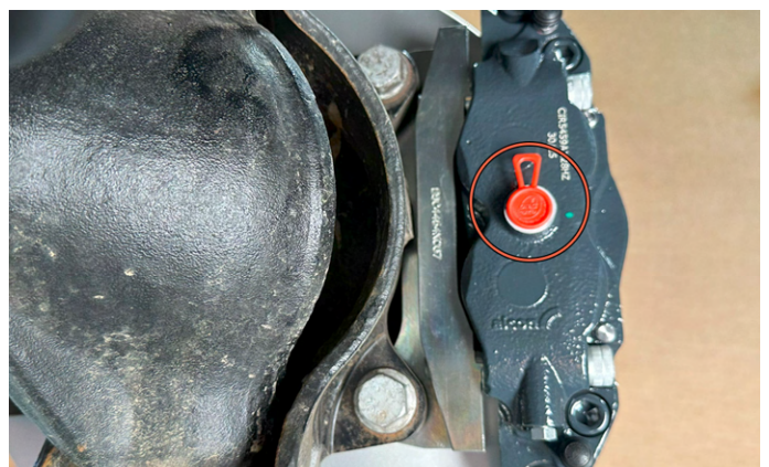
12. Remove the caliper brake line port cap.
