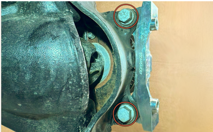
9. Apply a few drops of blue threadlocker and then torque to 120 ft lbs.
