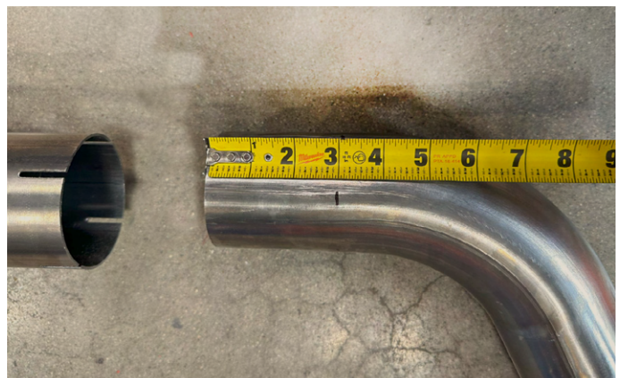
20. To facilitate assembly, mark the 3" slip pipes at 3 inches.
