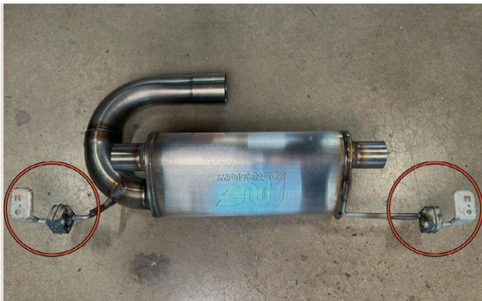
19. Install the removed hangers onto the muffler assembly as shown.
