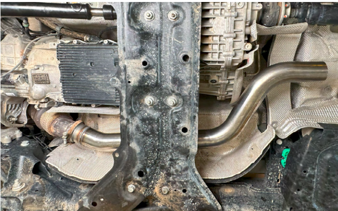
21. Install the inlet pipe assembly onto the front collector and reinstall the clamp nut and bolt assembly. Hand tighten only.
