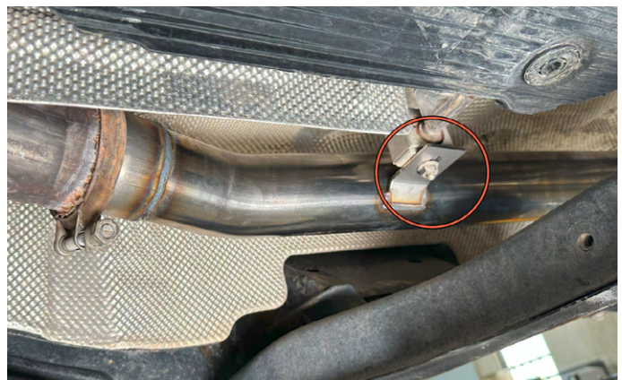
22. Reinstall the center hanger nut. Hand tighten only.
