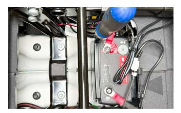
**3.** Use a T15 Torx bit to remove the four battery charger bolts.
