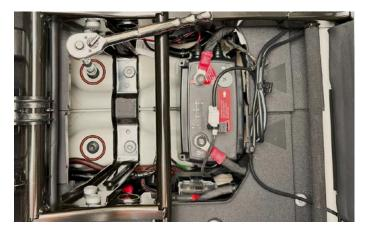
**Z.** Use a T50 Torx bit to remove the two black button head bolts as shown.
