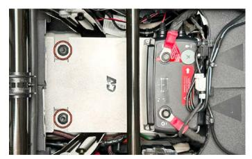
**5.** Install the two factory button head bolts at the front of the accessory plate. Hand tighten only. Use the four supplied M4 bolts to bolt down the CTEK battery charger. Fully tighten all hardware. Torque the two front button head bolts to 30 ft lbs and the M4 bolts to 23 in lbs.
