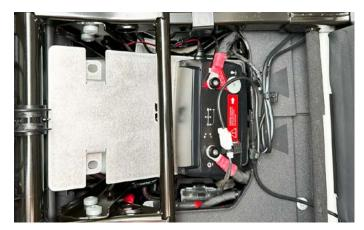
**4.** Install the AO accessory plate starting from the front of the seat base. Slide the accessory plate under the CTEK battery charger as shown.
