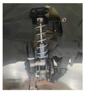
Fig. 20: Final FOX strut installation.
