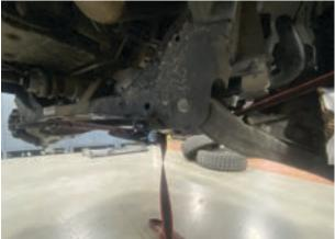
Fig. 4: Secure a ratchet strap on the hub end.
