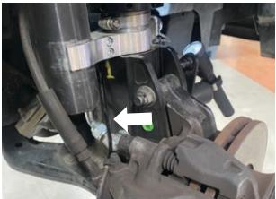
Fig. 19: Route the wire between the strut body and strut hose.
