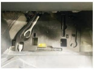
Fig. 7: Unclip the tool tray.
