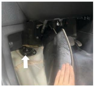
Fig. 10: Lift the footwell floormat to expose tophat bolts.
