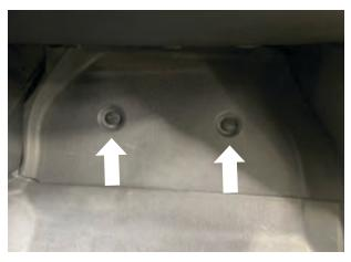
Fig. 6: Remove fasteners.
