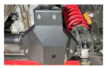
6. Fully tighten all 4 bolts. Torque the 4 M10 bolts to 31 ft/lbs.
