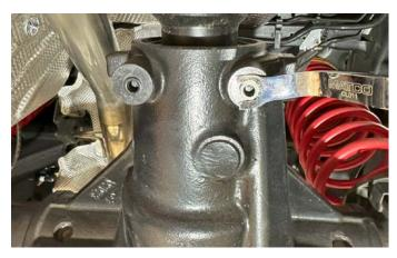
Z. Remove the thread caps using a panel clip removal tool or a pick.
