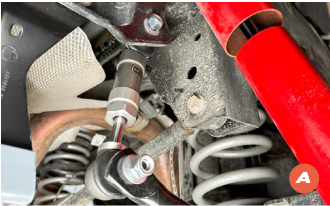
14 A/B. Install the Apex airLYNX starting at the upper mount. Install the supplied washers with the concave side towards the mount. The airLYNX must be installed with the Schraeder fill port facing forward. Use a 19mm open wrench and a 1/4" Allen wrench to fully tighten the link nuts. To tighten, rotate wrench and nut while holding stud with the Allen wrench. Torque to 30 ft lbs.
