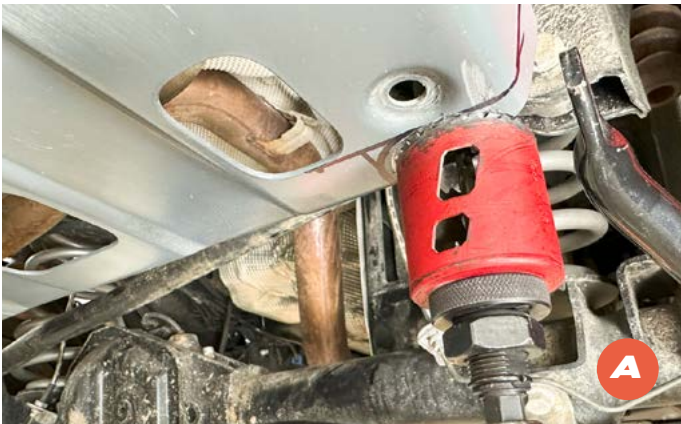
7 A/B. Use a 2" hole saw to drill through the corner of the skid plate. Drill only enough to make the radius.
