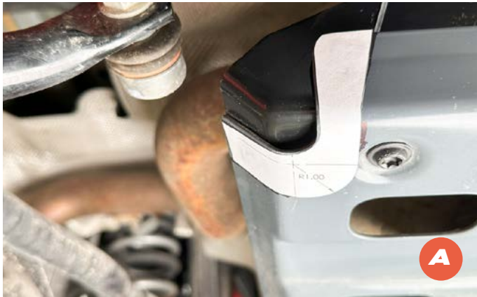
2 A/B. Use a marker and the supplied template to mark the skid plate cut location as shown.
