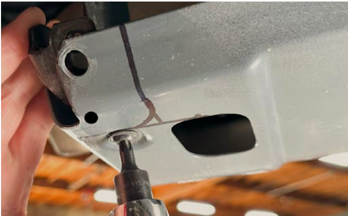
5. Use a T45 Torx bit to remove the skid plate to bracket bolt.
