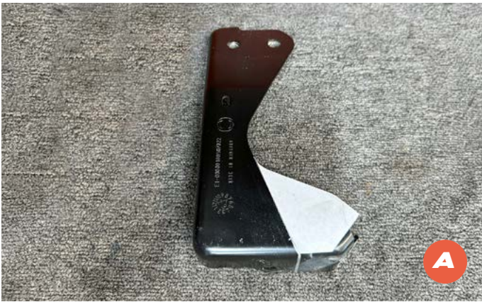
11 A/B. Use the supplied template to mark the front lower portion of the skid plate bracket.
