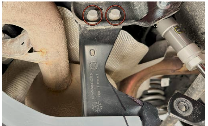
6. Use a 15mm wrench/socket to remove the two upper skid plate bracket bolts. Remove bracket.
