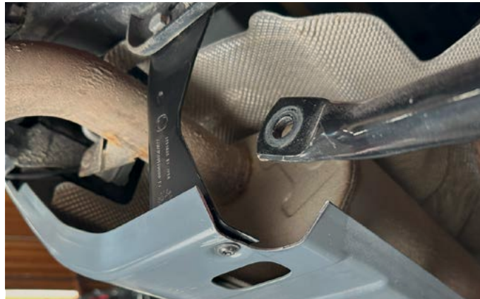
13. Re-install the skid plate bracket using the factory bolts.
