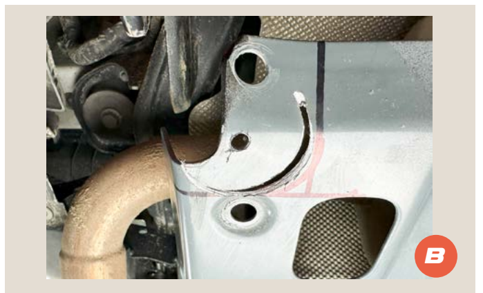
7 A/B. Use a 2" hole saw to drill through the corner of the skid plate. Drill only enough to make the radius.
