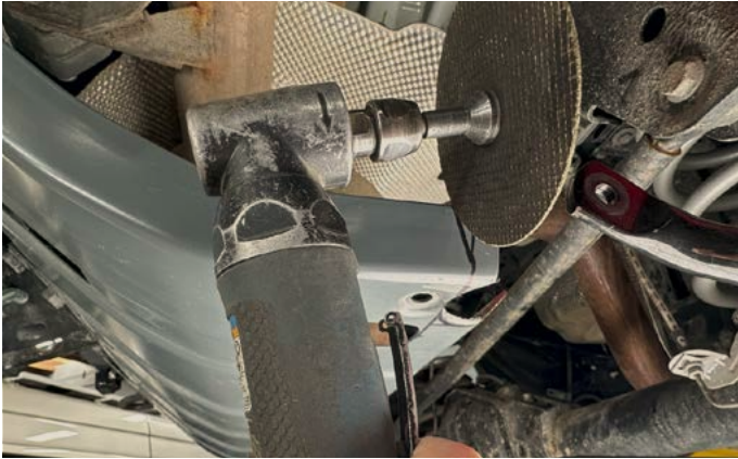
9. Use a cut-off wheel to cut from the side edge of the skid plate to the previous drilled radius.
