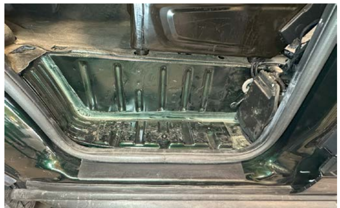
6. Use a 10mm socket/wrench to remove the three step molding bolts then remove molding.
