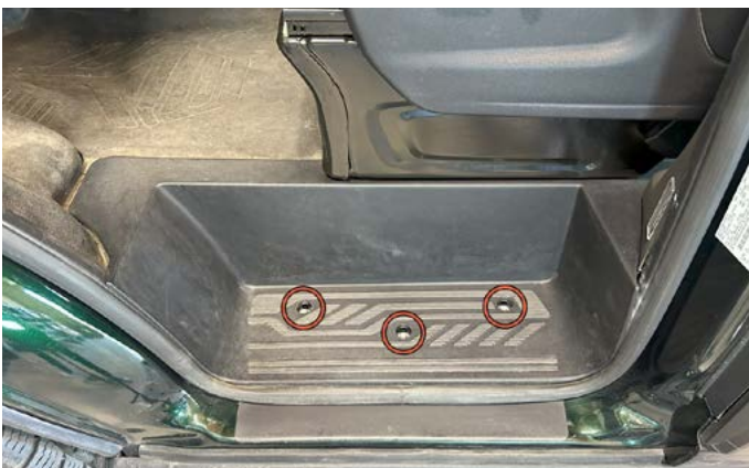
5. Remove the three screw caps from the step molding.
