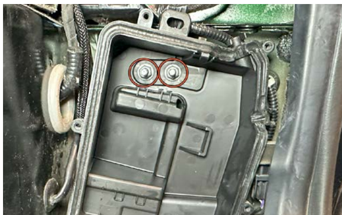
10. Remove module and then use a 10mm socket/wrench to remove the two module box nuts.
