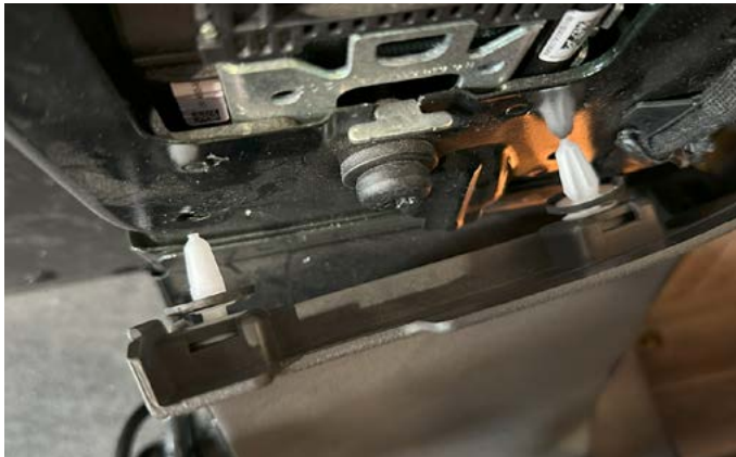
3. Use a clip removal tool to remove the lower B-Pillar molding.
