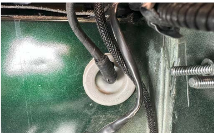
11. Remove the module box. With the module box removed, there is full access to the factory wire harness grommet.
