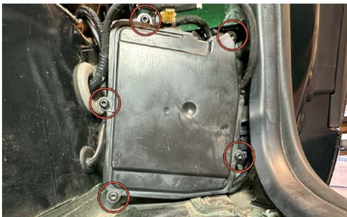
7. Use a T25 Torx bit to remove the five module screws.
