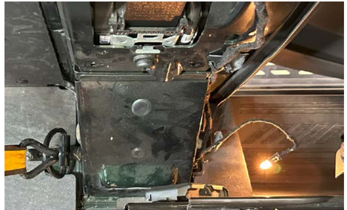
4. Remove the courtesy light from lower molding.
