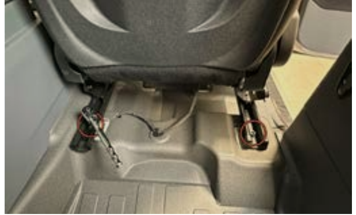
6. Slide seat forward. Use a T50 Torx bit to remove the two rear seat bracket bolts.
