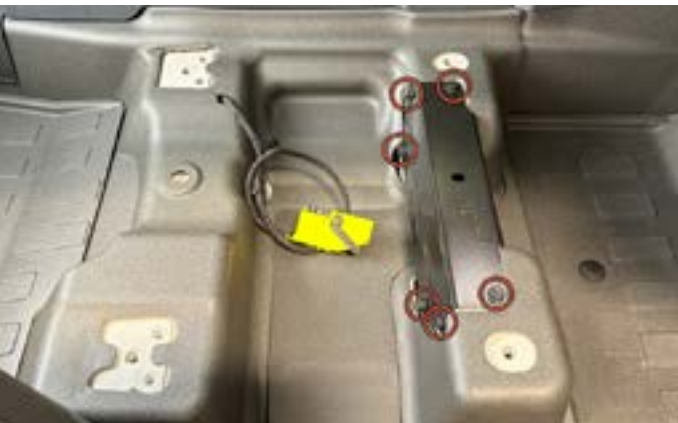
9. Carefully remove seat from vehicle. Use a 13mm socket/wrench to remove the six seat crossmember bracket screws. Save screws.
