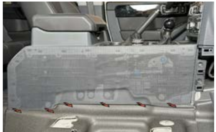
14. Pull out on the lower portion of the center console panel. Completely remove panel.
