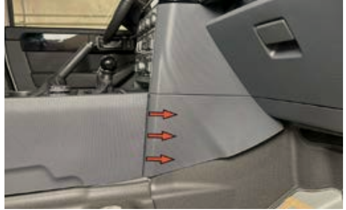
12. Pull out on front lower console molding. Only partial remove.
