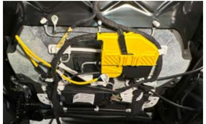
36. Re-connect the yellow seat harness to seat and re-attach harness clip to seat bottom. Follow steps 1-7 to re-install seat. Torque seat bolts to 19 ft/lbs.
