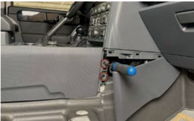
13. Use a T20 Torx bit to remove the two center console molding screws.
