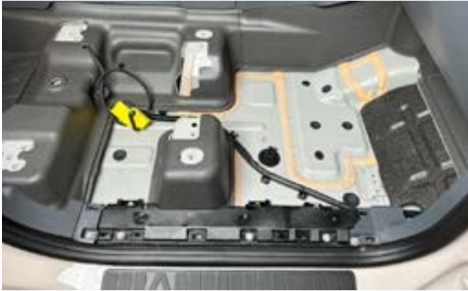
11. Remove center and front floor pads.
