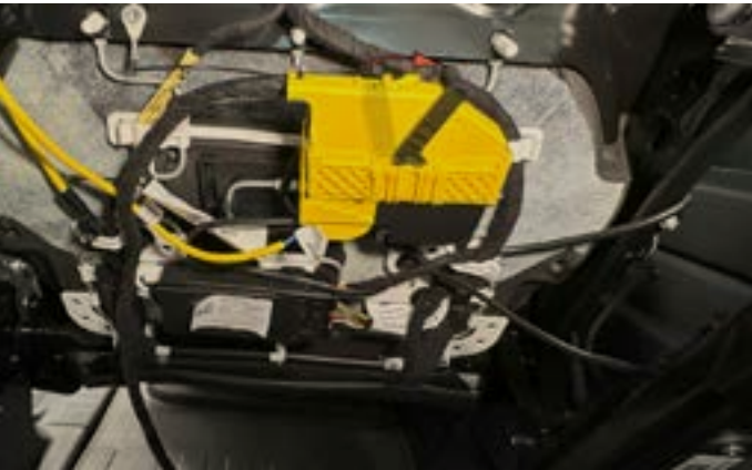
7. Lay seat back. Locate the yellow seat harness the plug. Push lever lock tab and rotate lever to the right. This will release harness connect plug from the seat. Note: Caution. While seat is disconnected, vehicle ignition must remain in the off position to avoid triggering the ABS warning light. The ABS light can only be cleared by an Ineos dealer.
