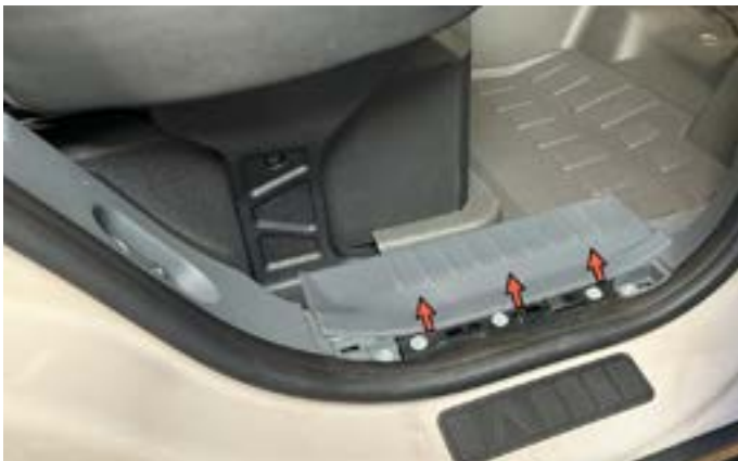
15. Pull up on rear door plastic edge molding and remove. Remove rear floor mat.
