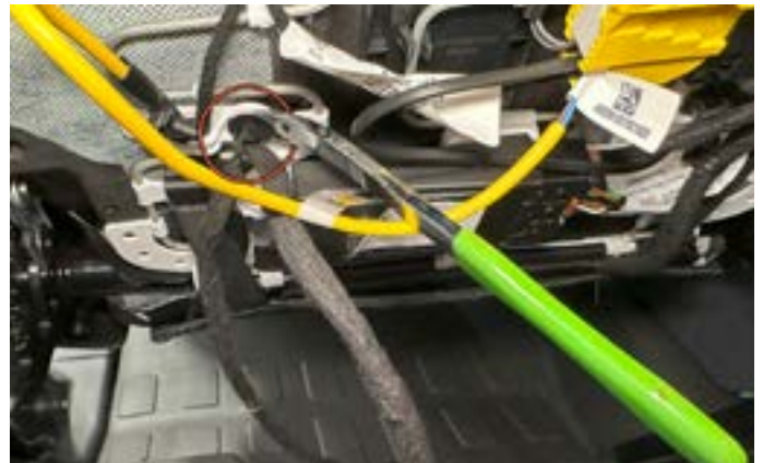
8. Use a clip removal tool to release seat harness clip from seat bottom.
