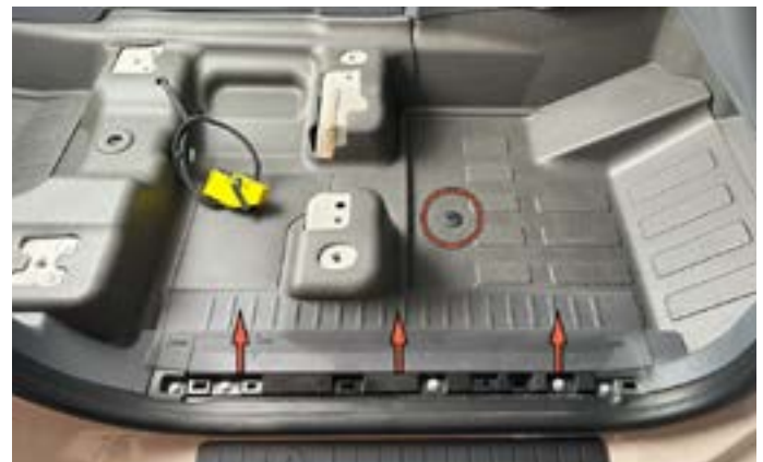
10. Pull up on plastic edge molding and remove. Loosen the front floor pad nut leave it.
