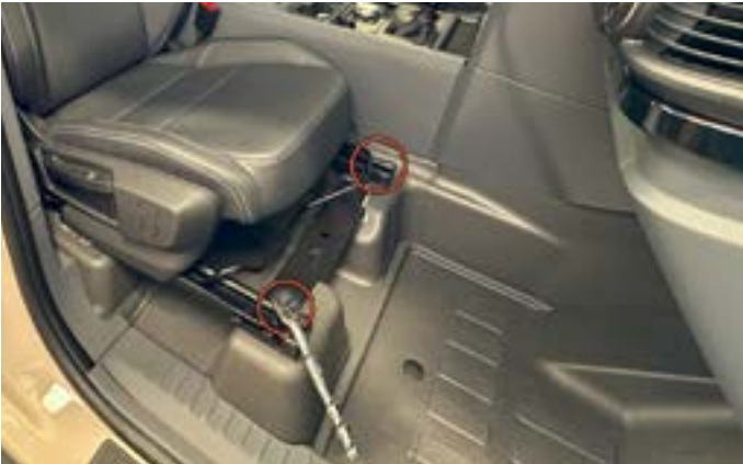
5. Slide seat back. Use a T50 Torx bit to remove the two front seat bracket bolts.
