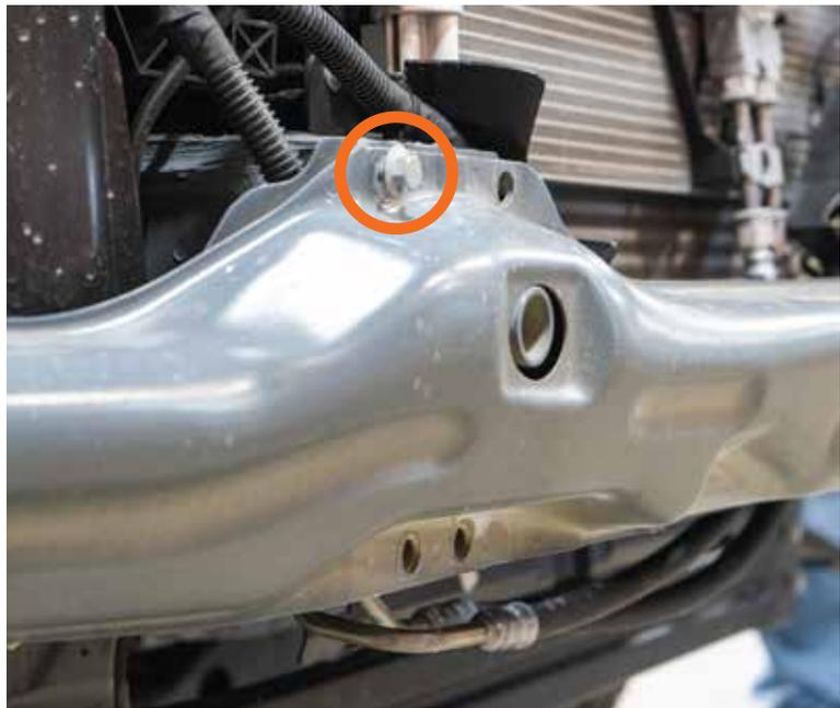
8. Remove the loosened bolt holding the crash bumper on the driver's side and install the driver's side AO Light Bar Bracket. Align the mounting holes with the crash bumper holes. Install the bracket and the crash bumper to the vehicle using an 8mm bolt removed earlier. Use red thread locking compound when installing the bolt. Do not fully tighten it yet. Repeat the process on the passenger's side of the vehicle.
