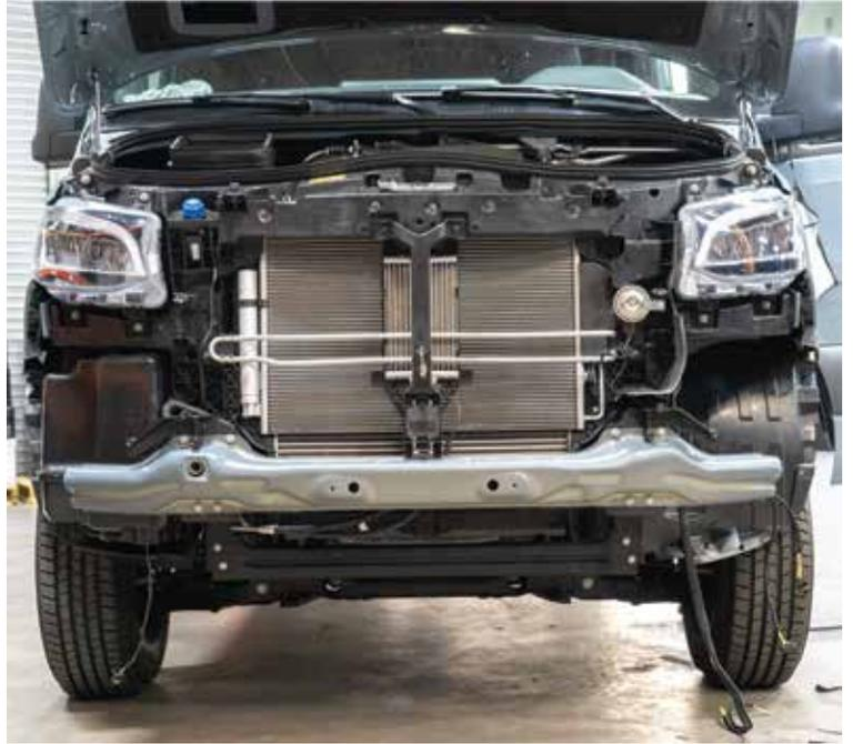
14. Reconnect the parking sensor & fog lights harnesses to the vehicle before installing the bumper cover. Use the 2 T-30 torx upper bumper bolts to keep the bumper in place. Do not fully tighten them yet. Push the bumper cover clips back into place, starting under the headlights and working out to the sides of the vehicle. Then fully tighten the 2 T-30 torx upper bumper bolts.
