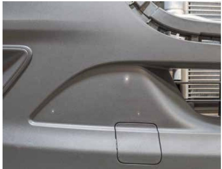
12. Remove the 2 T-30 torx upper bumper bolts and detach the bumper cover. Locate the 6 marking points from the locating pins on the inside of the bumper and drill small pilot hole through each marked point. Then, use a step bit to drill 7/8" holes for the Ferrata Light Bar.
