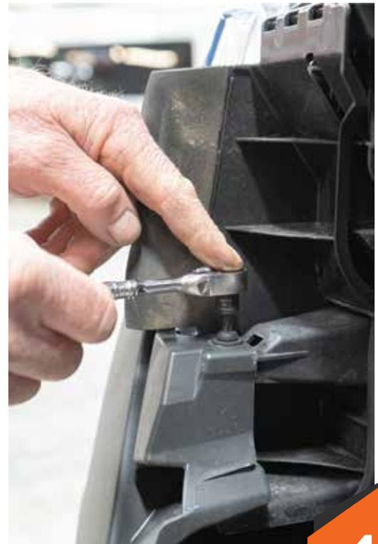
5. Remove the temperature sensor found on the top of the driver's side corner of the bumper cover. Use a T-45 torx to remove the 2 bolts in the front step. Pull along the edges of the bumper cover to remove it from the vehicle. Set the bumper cover aside.
