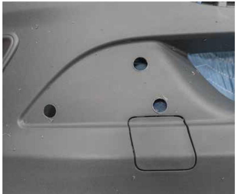
13. Insert the “t-shaped” DISTRONIC cruise control sensor bracket back into the crash bumper. Use the 2 T-25 Torx screws removed earlier to attach the top of the bracket into the vehicle.
