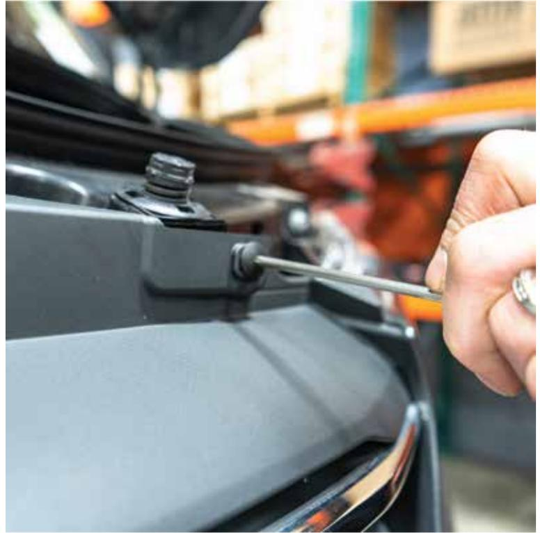
2. Pull firmly along the lower portion of the grille to remove it. Unplug the front camera by pushing in on the clip and gently pulling the cable from the back of the camera.
