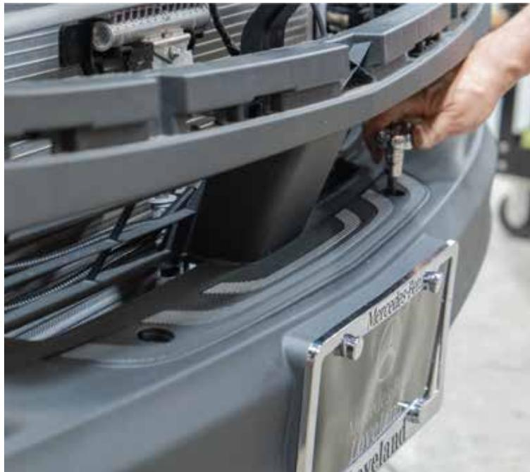
16. Use the 6 supplied 3/8" allen bolts, washers, and spacers to install the Ferrata light bar onto the bumper. Use red thread locking compound when installing the bolts.
