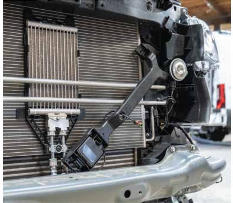
7. Use a 13mm socket to remove 3 out of 4 bolts holding the crash bumper on each side. Then loosen, but do not remove, the remaining 2 bolts holding the crash bumper.
