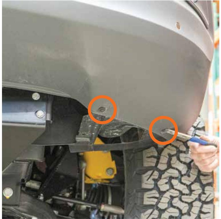
4. Use a T-30 torx to remove the 2 bumper bolts located next to the radiator support.
