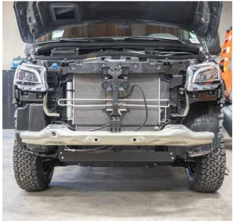
6. Remove the 2 T-25 Torx screws holding the “t-shaped” Distronic cruise control sensor bracket. Remove the bracket from the crash bumper and set it aside.
