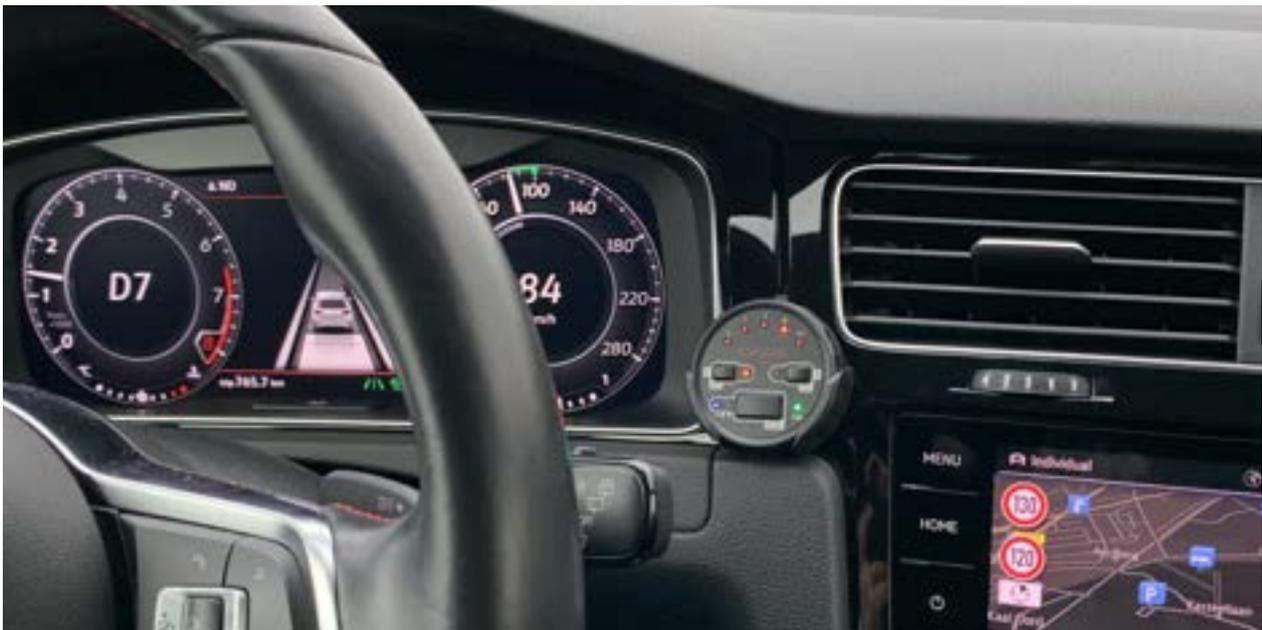
Test the stability of the wireless signal by starting the remote. If necessary rearrange the module or the remote.
