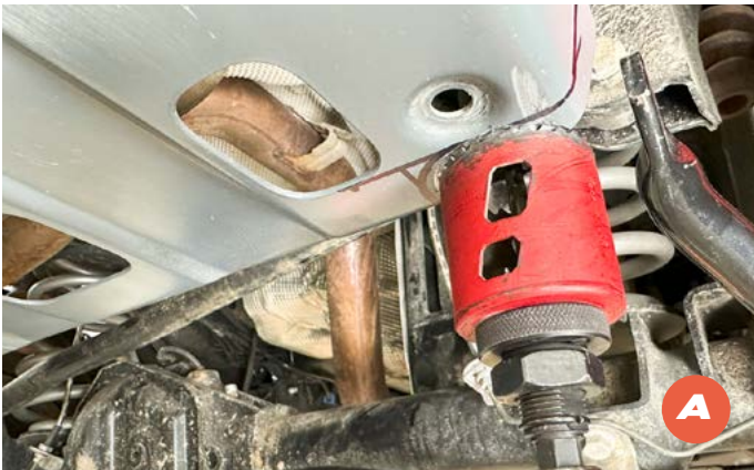
7 A/B. Use a 1 ½" hole saw to drill through the corner of the skid plate. Drill only enough to make the radius.
