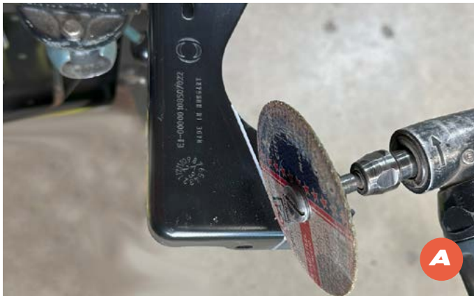
12 A/B. Use a cut-off wheel to cut the bracket at the marked line. Sand the cut edges and then apply a coat of preventative paint.
