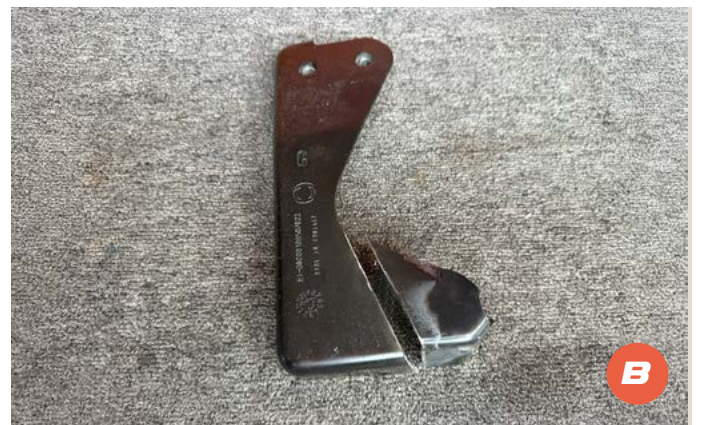
12 A/B. Use a cut-off wheel to cut the bracket at the marked line. Sand the cut edges and then apply a coat of preventative paint.
