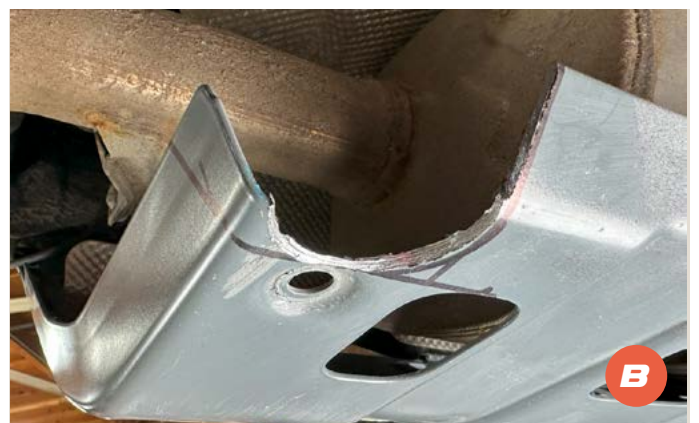
8 A/B. Use a cut-off wheel to cut from the back edge of the skid plate to the previous drilled radius.
