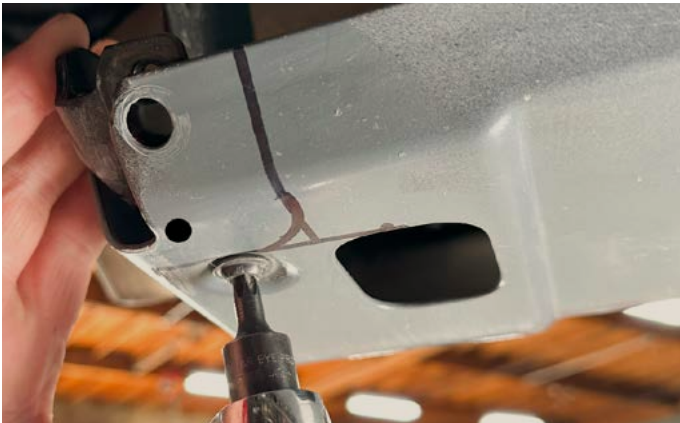
5. Use a T45 Torx bit to remove the skid plate to bracket bolt.
