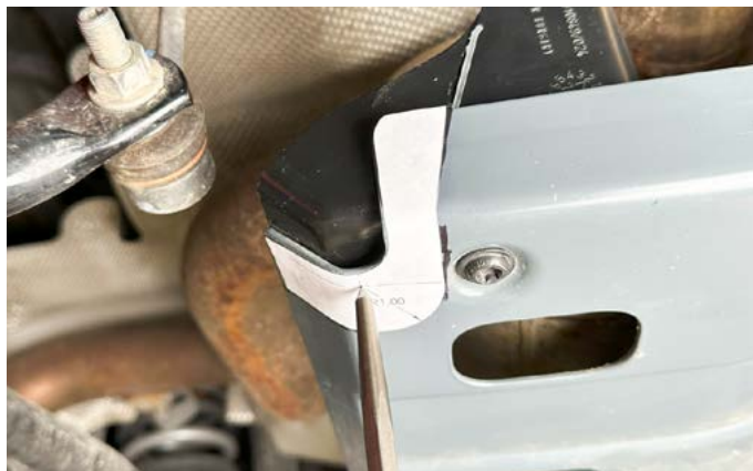
3. Use a center punch to mark the skid plate using the template as the guide.
