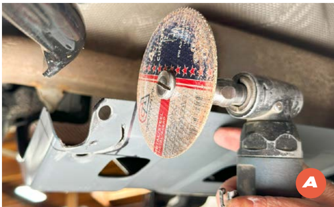
8 A/B. Use a cut-off wheel to cut from the back edge of the skid plate to the previous drilled radius.
