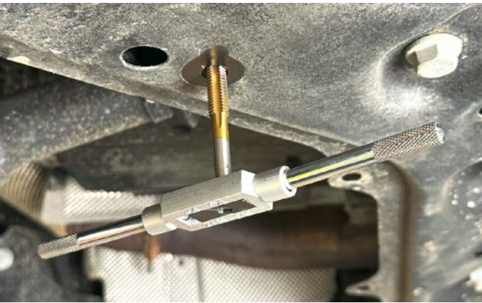
21. Clean the two factory threaded holes as necessary. Use a 10mm x 1.5mm tap to clean any damaged threads.
