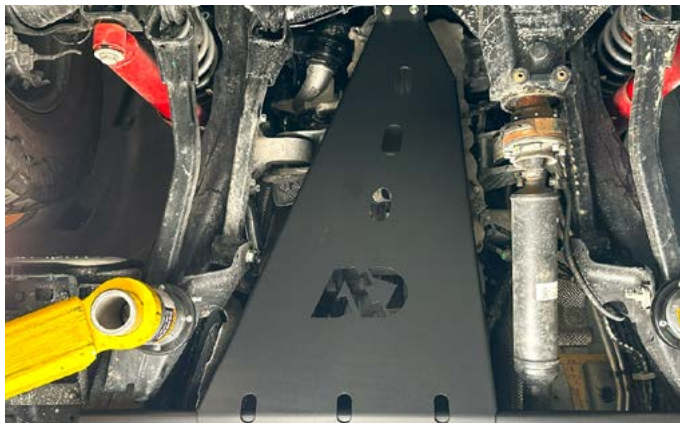
29. Fully tighten the four bolts and nuts. Torque to 37 ft lbs.
