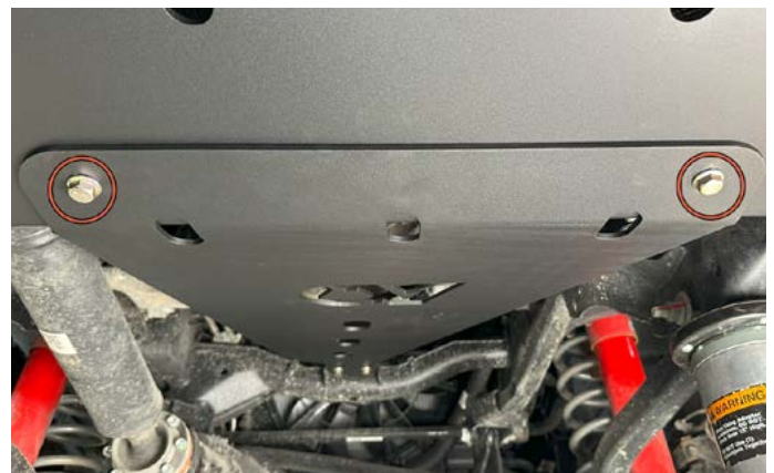
28. Bolt the engine skid plate to the AO Transmission/Transfer Case Skid Plate using two of the supplied M10 flange bolts and flange nuts.
