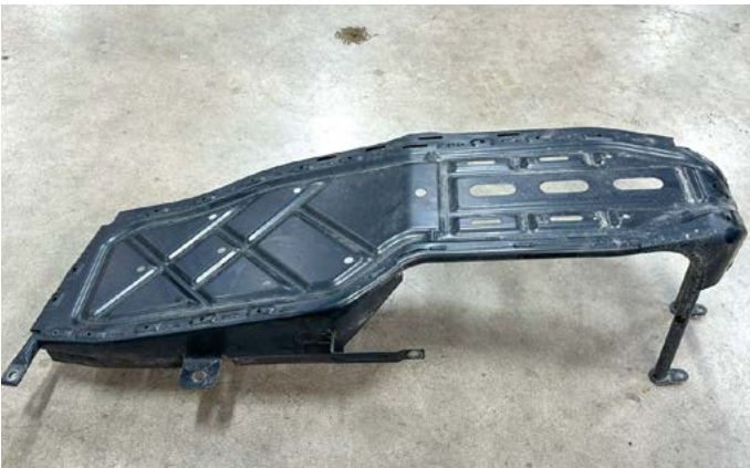
34. Place the factory fuel tank skid plate on the floor as shown.
