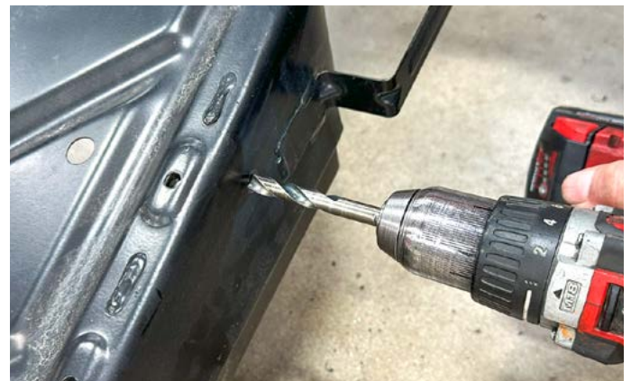
41. Drill a hole at all six marked locations using a \frac{5}{16} " drill bit.
