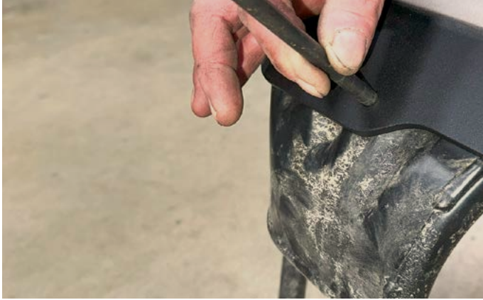
36. The AO skid plate has six holes around the sides. Use an \frac{11}{32} " center-locating punch to mark the drill location on all six holes onto the factory skid plate.
