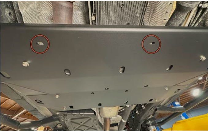
25. Locate the two slotted holes located on the AO Transmission/Transfer Case Skid Plate.
