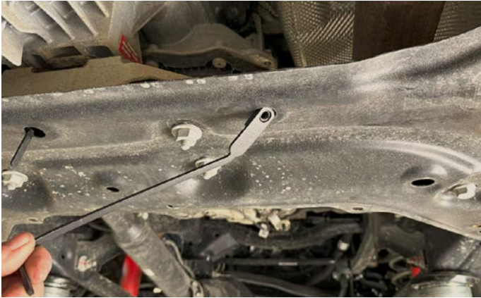
7. Insert the passenger side flag nut into the crossmember as shown..
