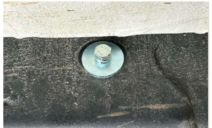
18. View from outside passenger frame rail of the frame support bracket bolt and washers. Do not fully tighten.
