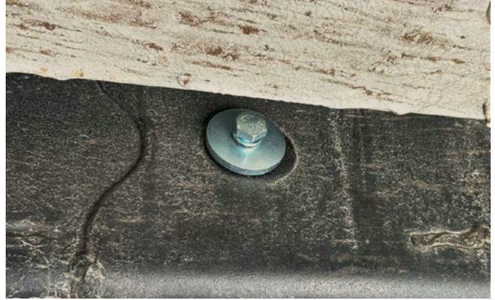
20. View from outside passenger frame rail of the frame support bracket bolt and washers. Do not fully tighten.
