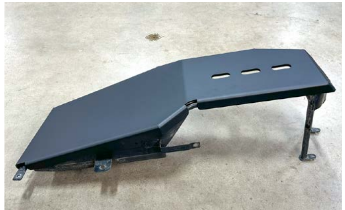
35. Place the AO Fuel Tank Skid Plate over the factory skid plate.
