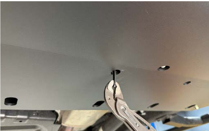
23. Use a pair of channel pliers to remove flag nut tabs.
