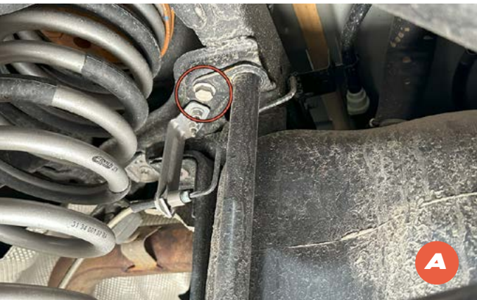
33 A/B. Use a 16mm wrench/socket to remove the two rear fuel tank skid plate mounting bolts.
