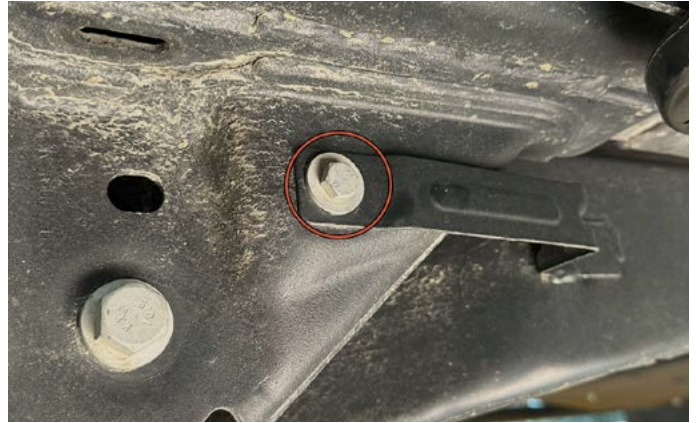
32. Use a 13mm wrench/socket to remove the side fuel tank skid plate mounting bolt.
