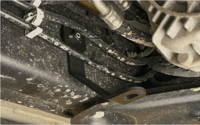
19. Install one of the supplied frame support brackets to the inside driver rail using the supplied M10 x 135mm hex bolt, large support washer, and M10 split lock washer.
