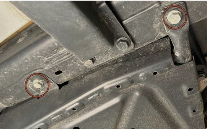
31. Use a 16mm wrench/socket to remove the two front fuel tank skid plate mounting bolts. Have a friend help hold skid plate.
