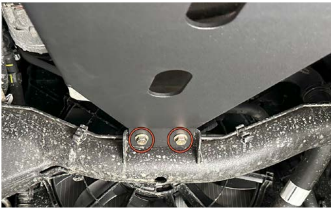
27. Bolt the engine skid plate to the front crossmember using two of the supplied M10 flange bolts and flange nuts.
