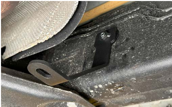
17. Install one of the supplied frame support brackets to the inside passenger rail using the supplied M10 x 135mm hex bolt, large support washer, and M10 split lock washer.
