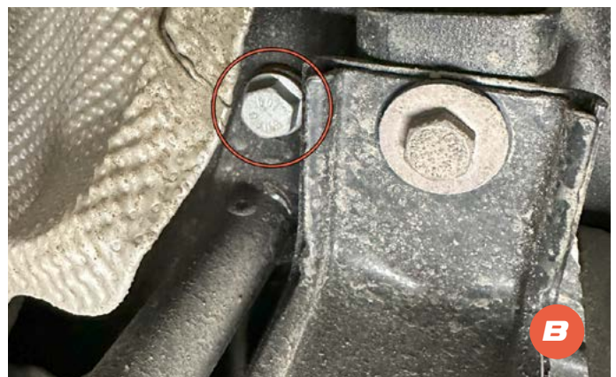
33 A/B. Use a 16mm wrench/socket to remove the two rear fuel tank skid plate mounting bolts.
