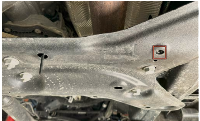
8. Align the flag nut threads with the outside 16mm crossmember hole as shown.
