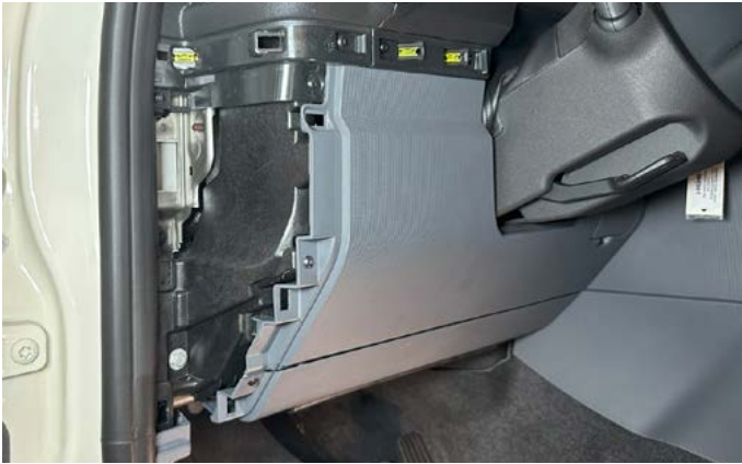
21. Pull out on the left corner dash panel and remove.
