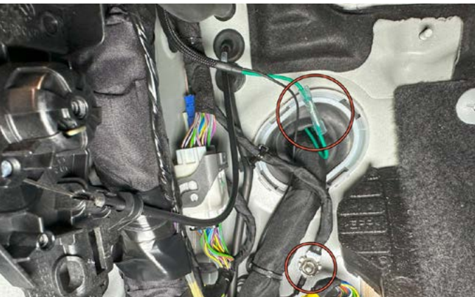
34. Attach the green dimmer wire to the Baja Designs green dimmer wire. Use a 10mm socket/wrench to attach the black ground wire ring terminal to the factory ground post. Use wire ties to secure switch harness.
