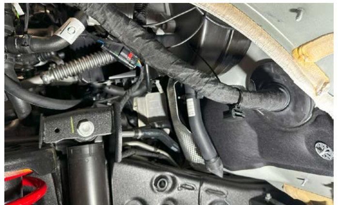
12. Re-wrap the harness using the previously removed harness tape. Use a zip tie to re-install to the the factory harness clip
