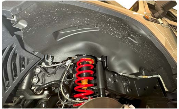
14. Re-install the fender liner, fender flare, mud flap, and wheel. **Retorque Wheel to Factory Specs**
