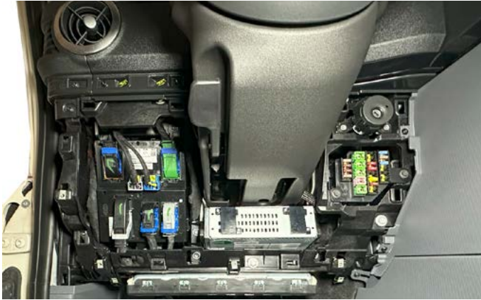
25. Pull out on the center dash panel and remove.
