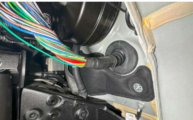
11. Re-install the grommet onto the firewall. Make sure the grommet is completely clipped onto the firewall.
