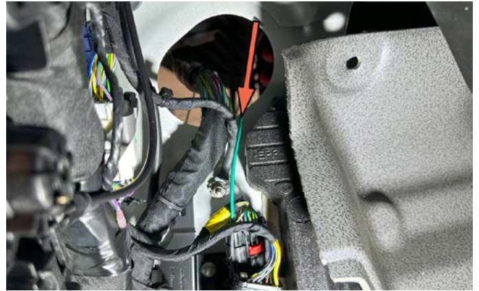
10. Run the green dimmer ground wire into cab.
