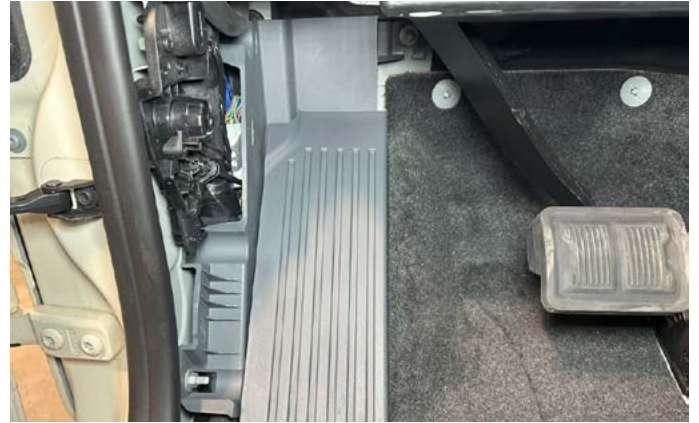
26. Pull out on the side kick panel and remove.
