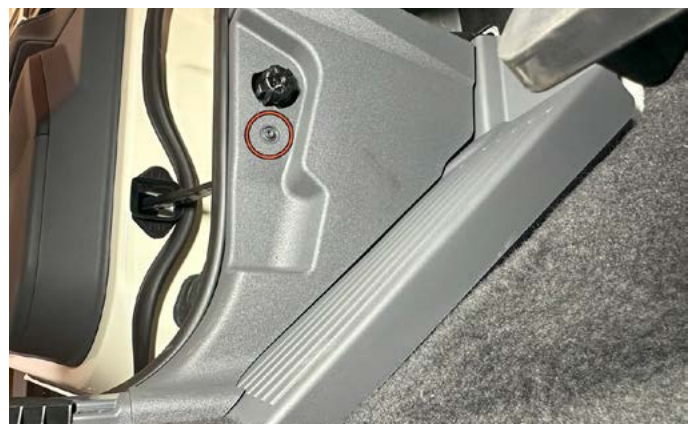
18. Use a T25 Torx bit to remove the kick panel screw.
