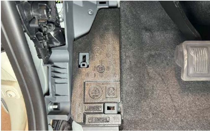
27. Pull up on the footrest panel and remove.
