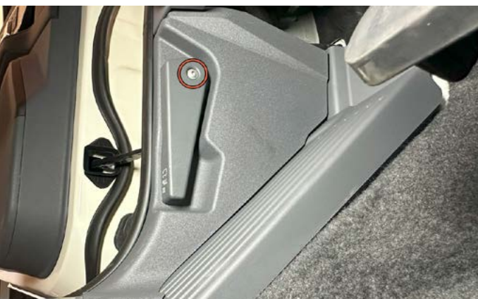
17. Use a T25 Torx bit to remove the hood latch release handle screw and remove handle.
