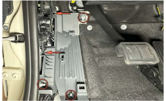
28. Remove footrest foam. Use a 10mm socket/wrench to remove the three footrest panel nuts and a T25 Torx bit to remove the two screws. Remove the lower footrest panel.
