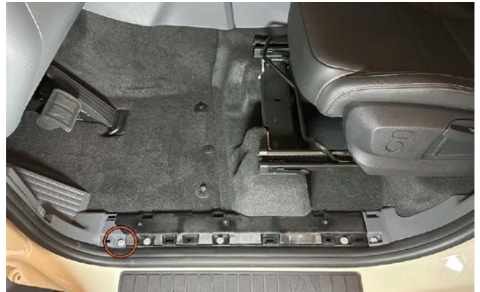
16. Pull up on the door sill panel and remove. Use a 10mm socket/wrench to remove rear kick panel bolt.
