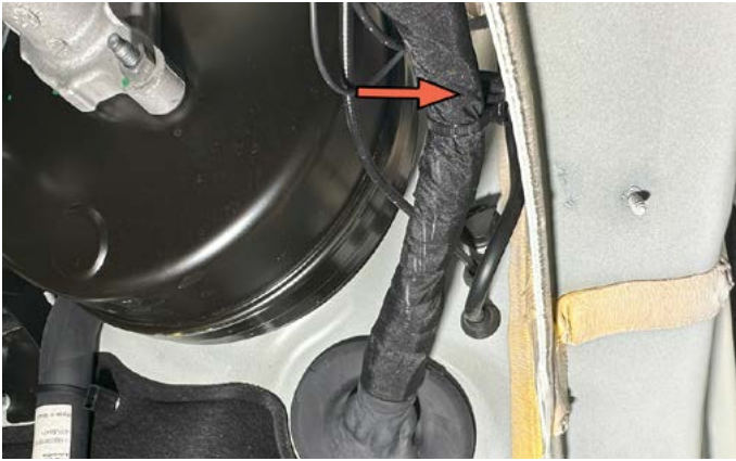
13. Re-attach the harness clip to the fender stud.
