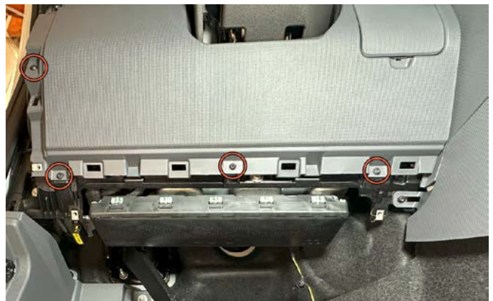
24. Use a T20 Torx bit to remove the four center dash panel screws.
