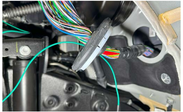
8. Unclip harness grommet from the firewall. Run the Baja Designs green dimmer ground wire through the grommet.
