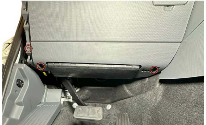
22. Use a T20 Torx bit to remove the three lower dash panel screws.
