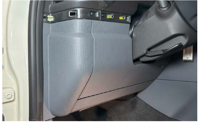
20. Pull out on the upper dash panel trim and remove.
