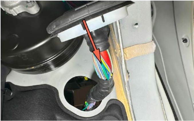
9. Run the green dimmer ground wire into the factory harness under the electrical tape. Remove and then replace the electrical tape if necessary.
