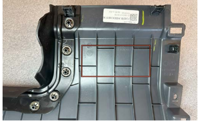
31. Carefully remove adhesive backed insulation.
