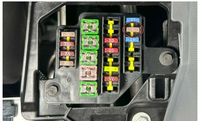
35. Remove the 5-Amp fuse from the left fuse bank.
