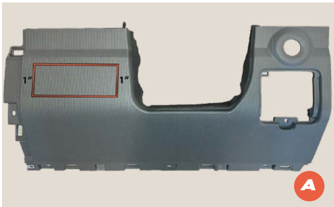
29. Recommended switch location shown. Before drilling hole into center dash panel, make sure there is enough room to clear the switch depth of approx. 3".
