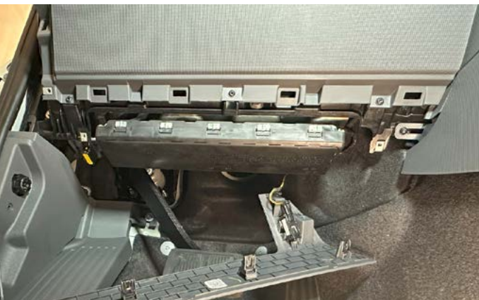
23. Pull out on panel and remove. Note: It is not necessary to unplug and remove the panel completely.
