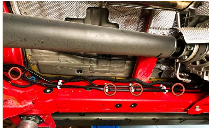
14. Secure the tubing to the existing brake line as shown.
