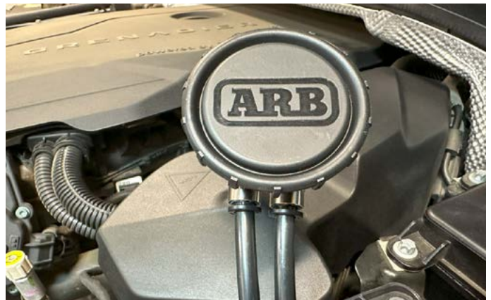
16. Cut the tubing at the master cylinder location leaving enough slack to properly install the filter and manifold assembly.
