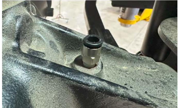
8. Install one of the supplied 1/8" BSP push in fittings. Use a 13mm deep socket to tighten fitting.
