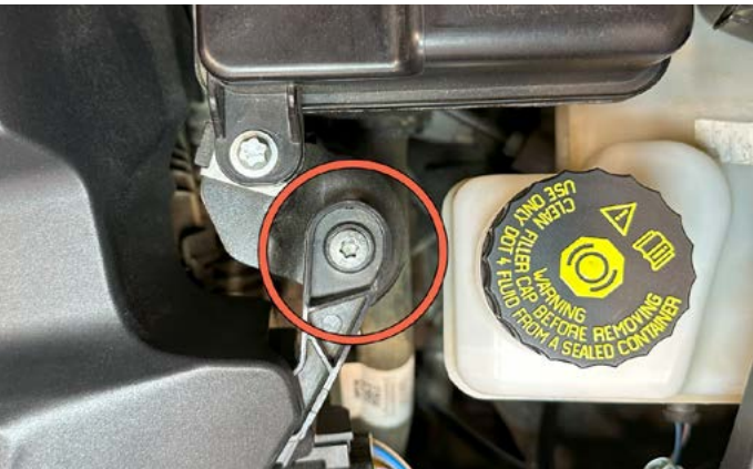
17. Use a T30 Torx bit to remove the bolt next to the master cylinder.
