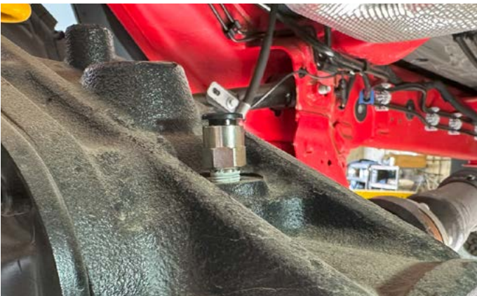
11. Rear Axle: The factory differential breather is located on the passenger's side of the center section. Use a 14mm deep socket to remove the factory breather. Clean the threads as necessary and install one of the supplied 1/8" BSP push in fittings. Use a 13mm deep socket to tighten fitting.
