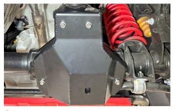
6. Fully tighten all 4 bolts. Torque the 4 M10 bolts to 40 ft/lbs.
