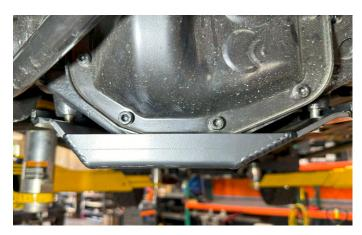
4. Install the AO Diff Skid Plate using the supplied (4) M10-1.5x20mm Start by adding a small drop of the supplied blue threadlocker to each bolt then install each bolt 2-3 turns only.
