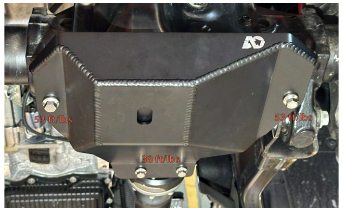
6. Fully tighten all 4 bolts. Torque the (2) M10 bolts to 40 ft/lbs and the (2) M12 bolts to 53 ft/lbs.
