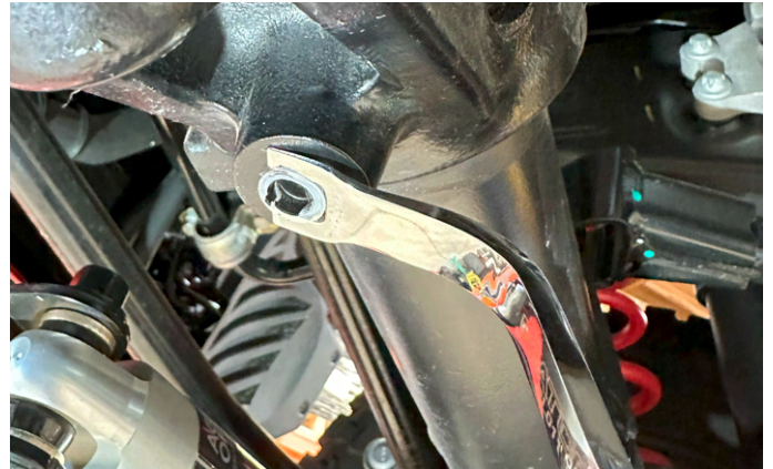
2. Remove the thread caps using a panel clip removal tool or a pick.
