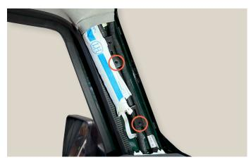
4. Remove the panel by pulling straight back. Note: The a-pillar comes from the factory with existing thread bosses.
