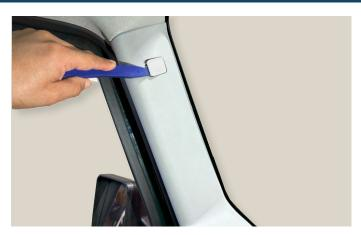
**Z.** Use a panel removal tool to remove the a-pillar screw cover.
