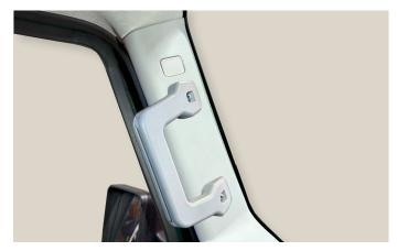
Install the AO A-Pillar Grab Handle using the supplied 6mm bolts. Torque to 4 ft/lbs.
