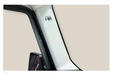
3. Use a T30 Torx bit to remove the panel screw.
