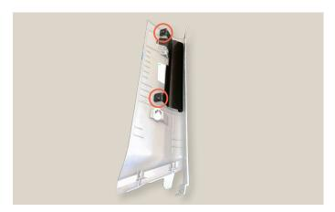
**5.** Use a T20 Torx bit to remove the rear panel support bracket off the a-pillar panel.
