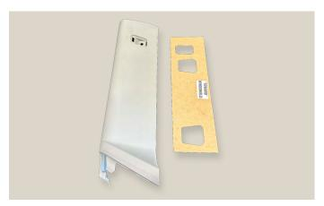
**7.** Position the supplied template. **Note: The template is labeled** "Toward Windshield". Toward Windshield side must be lined up on the a-pillar panel windshield edge.
