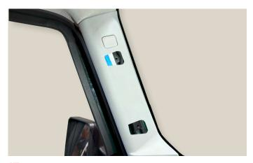
Re-install the a-pillar panel using the factory screw. Re-install the screw cover.
