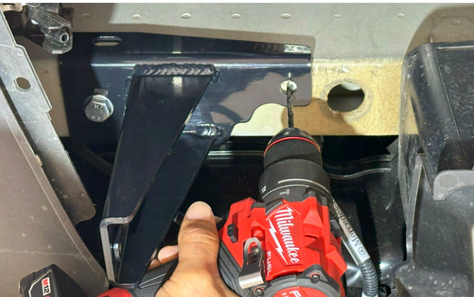
5. Use a 1/8" drill bit to make a pilot hole at the previously marked location.
