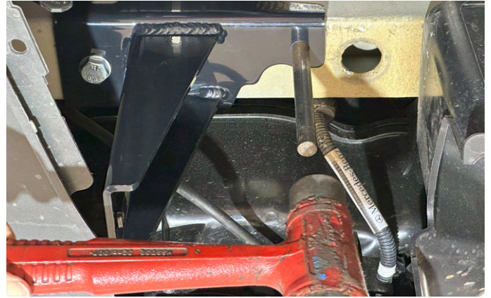
4. Use a 1/2" center-locating punch to mark the rear drill location.
