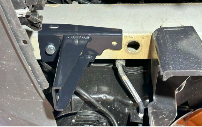
3. Install the AO Skid Plate Impact Bracket using one of the supplied 12mm X 1.50 bolts and washer. Install bolt through the front hole of bracket and into the factory threaded insert.
