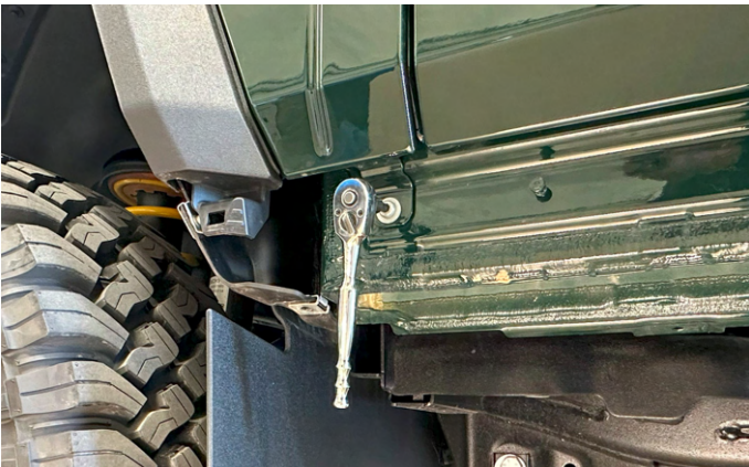
8. Use a T30 Torx bit to remove the lower front fender screw.
