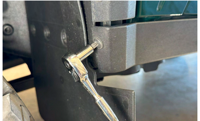
2. Use a T40 Torx bit to remove the screw at the front of the rocker panel molding.
