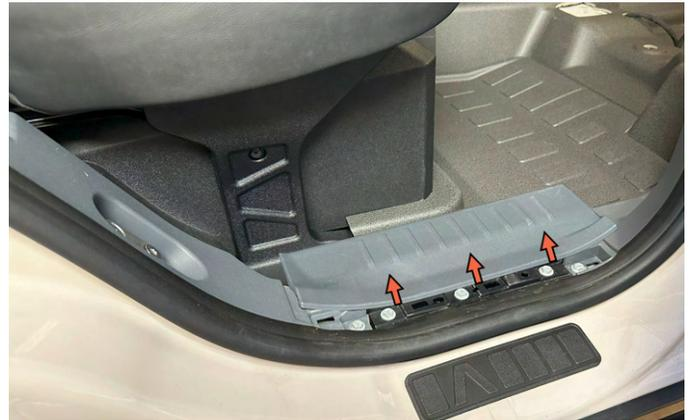
**15.** Pull up on rear door plastic edge molding and remove. Remove rear floor mat.
