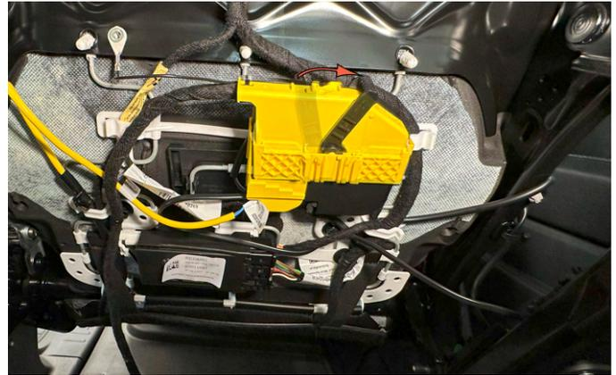
**7.** Lay seat back. Locate the yellow seat harness plug. Push lever lock tab and rotate lever to the right. This will release harness connect plug from the seat. **Caution. While seat is disconnected, vehicle ignition must remain in the off position to avoid triggering the ABS warning light. The ABS light can only be cleared by an Ineos dealer.**
