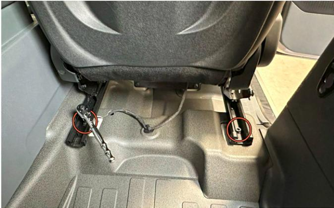
**6.** Slide seat forward. Use a T50 Torx bit to remove the two rear seat bracket bolts.
