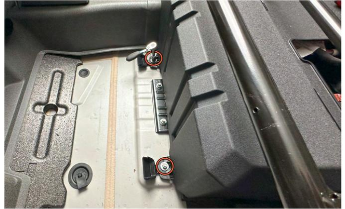
**25.** Use a 10mm socket to remove the two lower seat base panel nuts. Remove front panel.
