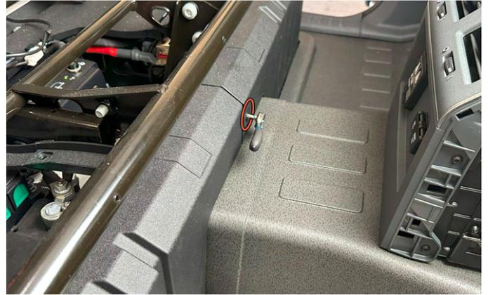
**19.** Use a T25 Torx bit to remove the front center lower seat base panel screw.
