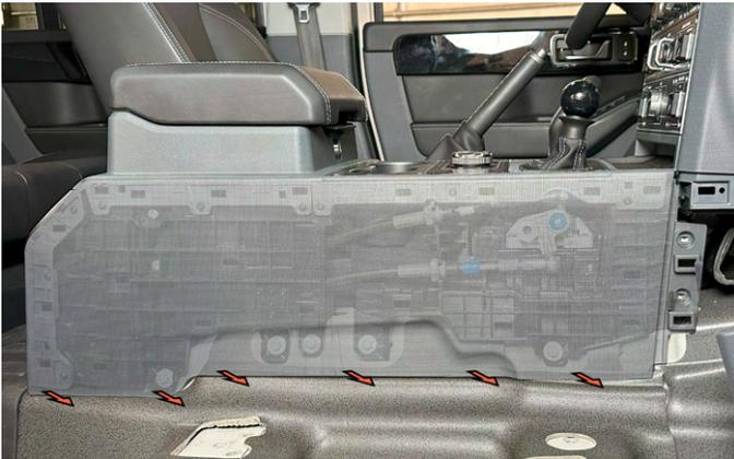
**14.** Pull out on the lower portion of the center console panel. Completely remove panel.
