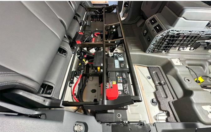
**22.** Remove rear lower seat panel from top of seat base frame.
