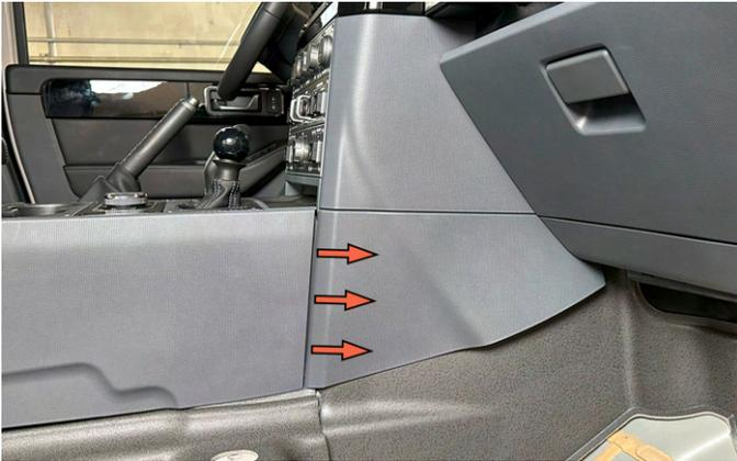
**12.** Pull out on front lower console molding. Only partial remove.
