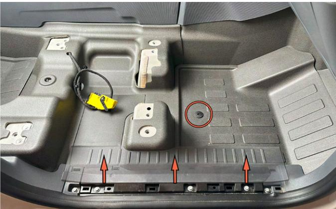
**10.** Pull up on plastic edge molding and remove. Loosen the front floor pad nut.
