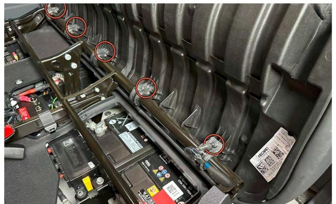
**17.** Use a T30 Torx bit to remove the five lower rear seat cushion brackets. Completely remove cushions.
