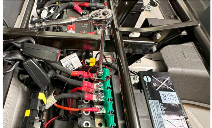
**31.** Remove the Littelfuse power distribution cover. Use a 13mm socket/wrench to remove the nut off the battery cable stud as shown.
