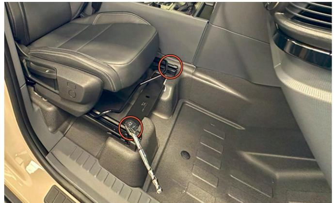
**5.** Slide seat back. Use a T50 Torx bit to remove the two front seat bracket bolts.
