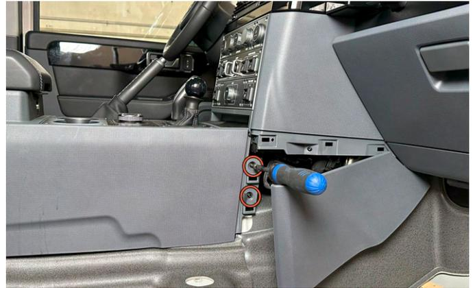
**13.** Use a T20 Torx bit to remove the two center console molding screws.
