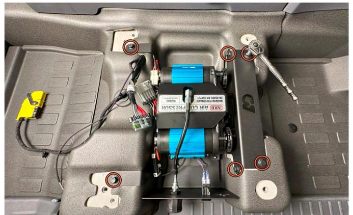
**39.** Install the AO Twin Compressor Assembly using the screws removed in step 10. Torque to 19 ft/lbs.
