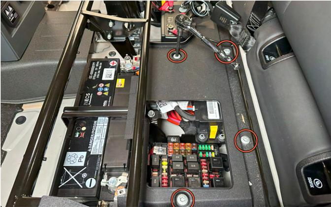
**26.** Use a T50 Torx bit to remove the four lower seat base panel screws.
