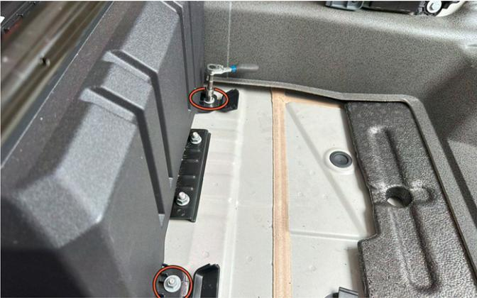
**20.** Use a 10mm socket to remove the two lower seat base panel nuts. Remove front panel.
