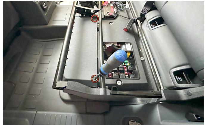
**23. Driver side:** Use a T25 Torx bit to remove the two lower seat base panel screws.
