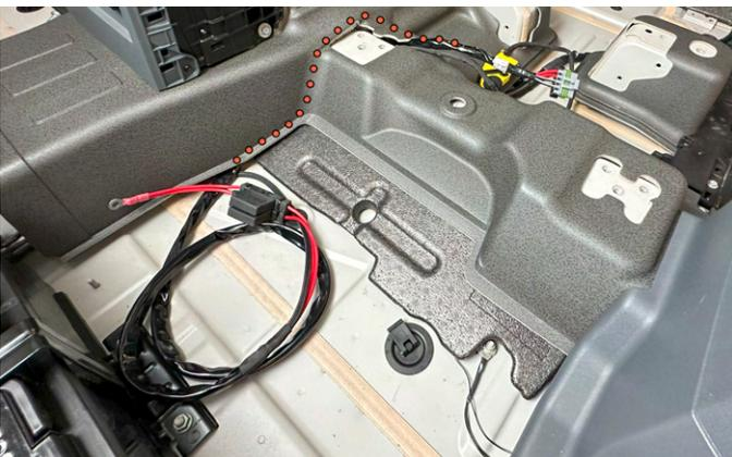
**28.** Route the power supply harness and the switch harness under the passenger side floor mat as shown.
