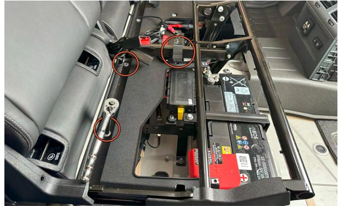
**21.** Use a T50 Torx bit to remove the two lower seat base panel screws. Unlatch panel at center of seat frame.
