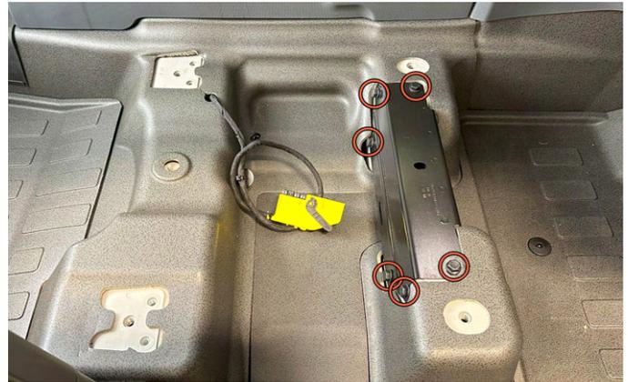
**9.** Carefully remove seat from vehicle. Use a 13mm socket/wrench to remove the six seat crossmember bracket screws. Save screws.
