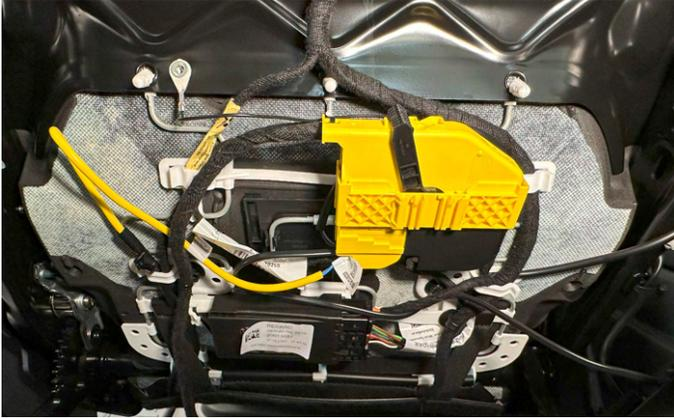
**42.** Re-connect the yellow seat harness to seat and re-attach harness clip to seat bottom. Follow steps 1-6 to re-install seat. Torque seat bolts to 19 ft/lbs.
