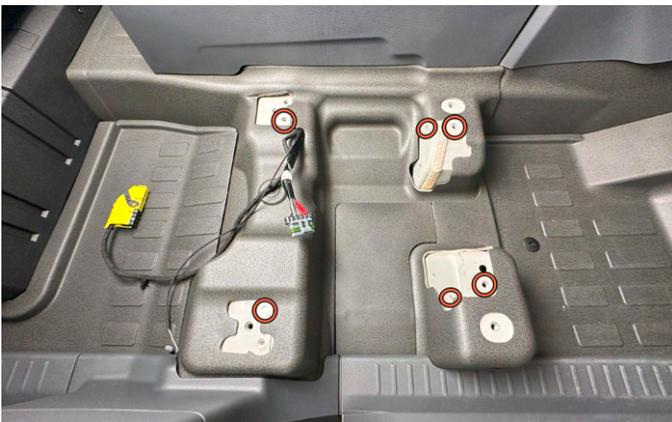
**38.** The AO Dual Compressor Assembly installs using existing factory thread holes. Remove the clear sticks found on the rear thread holes.
