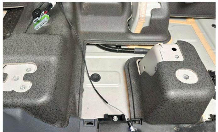
**29.** Leave approximately 18" of the switch harness wire exposed and approximately 5" of the power supply harness wire. Follow the same route as the existing factory seat harness wire.
