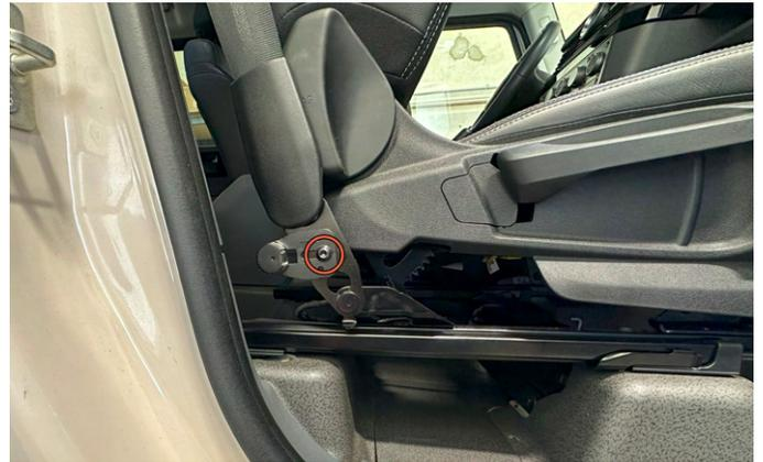
**3.** Use a T30 Torx bit to loosen the seat belt locking mechanism. Rotate mechanism 90 degrees.
