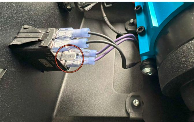
**40.** Locate the empty switch terminal as shown.
