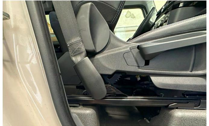
**2.** Slide lower rubber seat belt cover up to expose attachment point.
