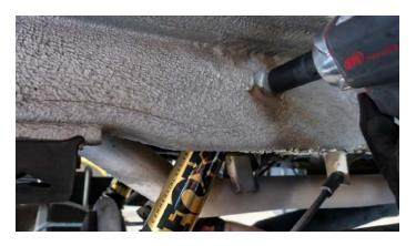
Apply thread-locker and install the upper shock hardware.
