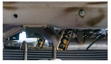
Torque upper shock bolt to 110 ft-Lbs. Torque lower shock bolt to 110 ft-Lbs.
