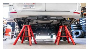
Lift vehicle and support vehicle with jack stands using factory jack points. Remove the rear wheels.
