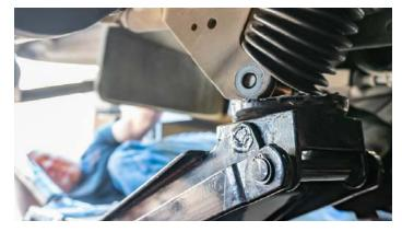
Use a jack to compress the shock. Line up the lower shock mount holes on the axle with the shock and install the shock bolt.
