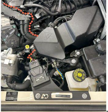
Install the supplied module bracket using the factory fender bolts with the supplied 1/4" spacers between bracket and fender. Attach the module to the bracket using the supplied 2" velcro pad and 2 wire ties.
