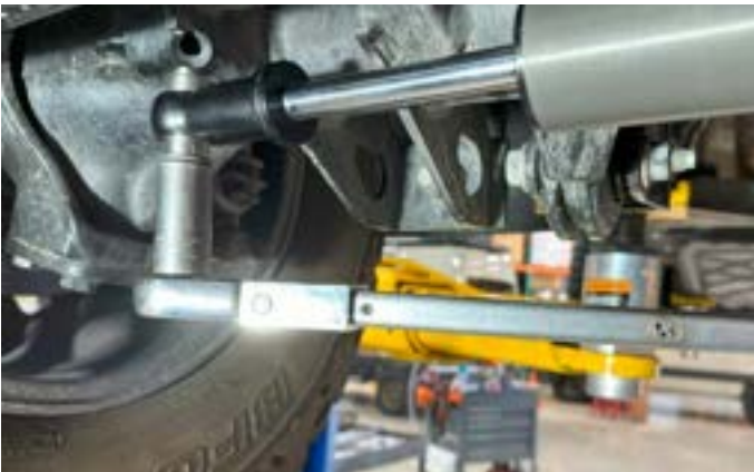
9. Fully tighten the passenger side bolt. Torque to 85 ft lbs.
