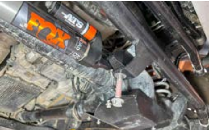
7. Line up the driver side stabilizer hole to the driver side mount holes and install the factory 14mm bolt.
