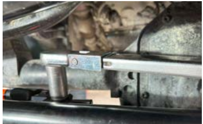
10. Fully tighten the driver side nut and bolt. Torque to 136 ft lbs.
