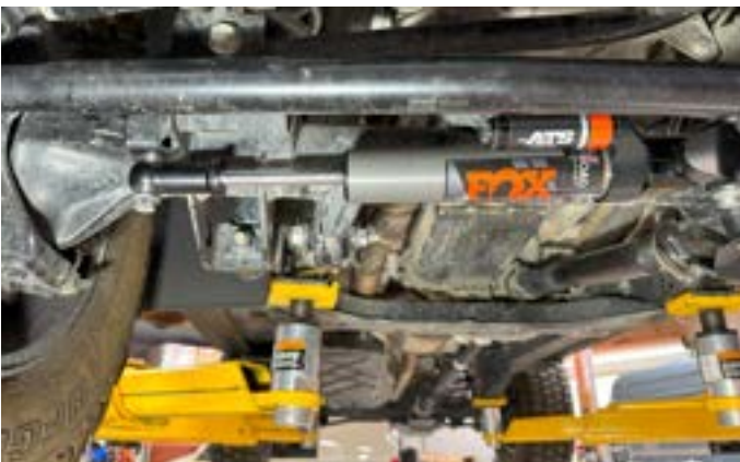
11. Turn the vehicle's wheels in both directions and check for any interference with any vehicle components.
