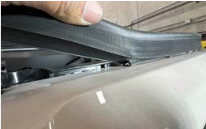
43. Start the weatherstrip installation from one end and work around until all t-clips are re-attached. Slide weatherstrip onto one end of t-clip then stretch weatherstrip and let it snap back until the clip is completely inserted in weatherstrip.
