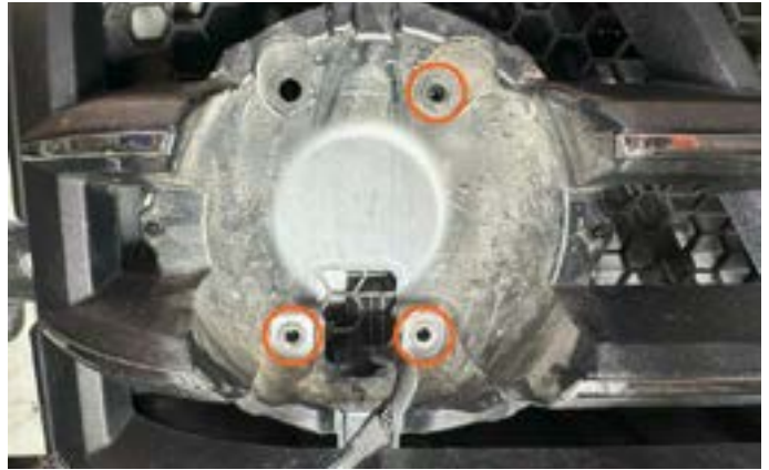
20. With the OEM fog lamp removed locate the 3 rubber grommets.
