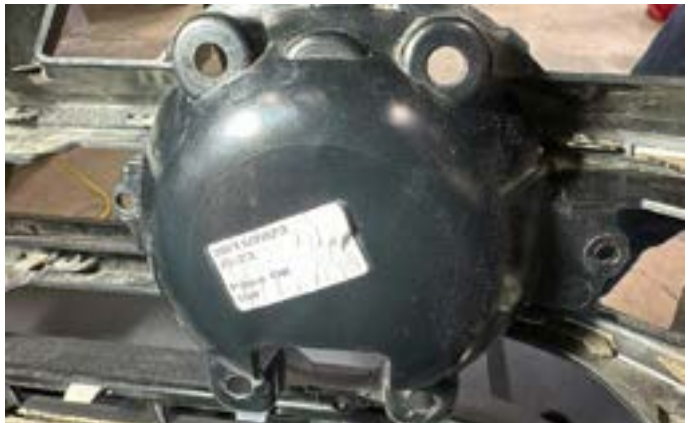
22. The fog lamp pocket is now ready for the new Agile Lamp Kit.
