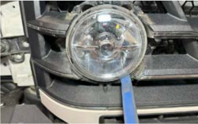
19. Use a plastic pry tool and starting from the bottom of the fog lamp pry the lamp straight forward.
