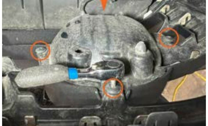
18. Use a T25 torx bit to remove the 4 fog lamp bezel ring screws.
