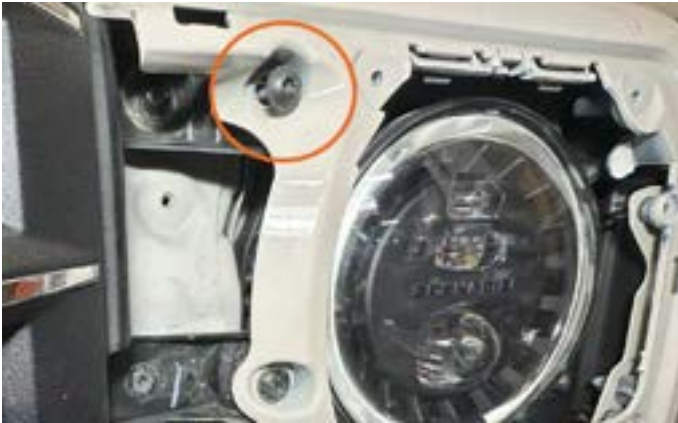
41. The extra-long T40 bolt goes in upper headlight panel.
