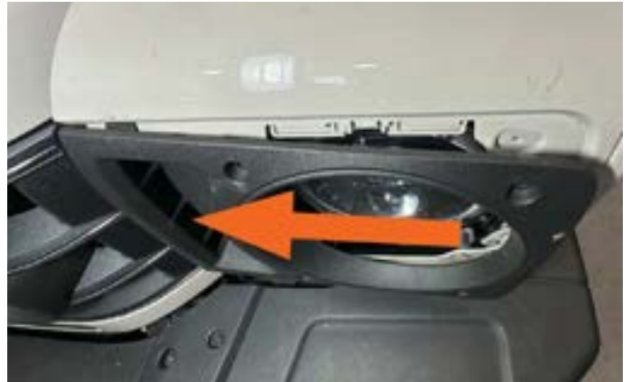
42. Come in at an angle when installing the headlight bezel then snap bezel into place.
