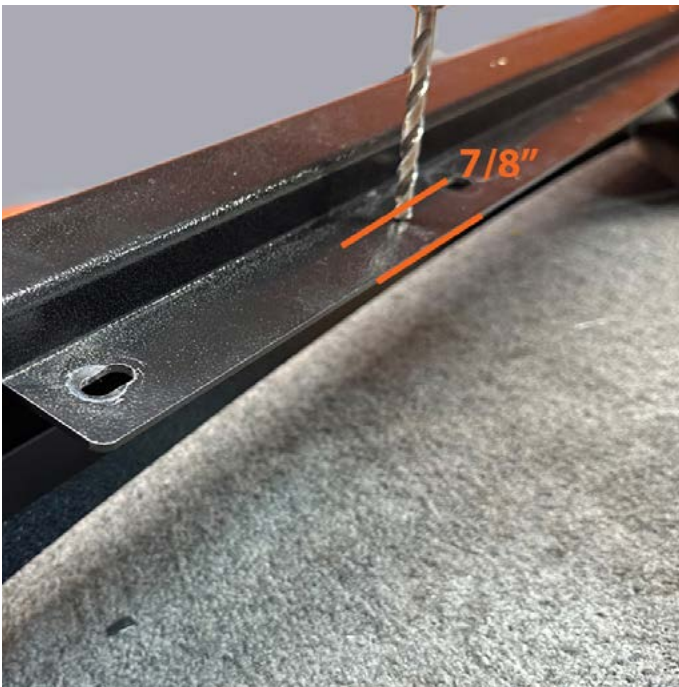
15. Locate the trace mark from step 11. Use an \frac{11}{32} \" drill bit and drilled at the center of the trace mark \frac{7}{8} \" from the inner edge of fairing.
