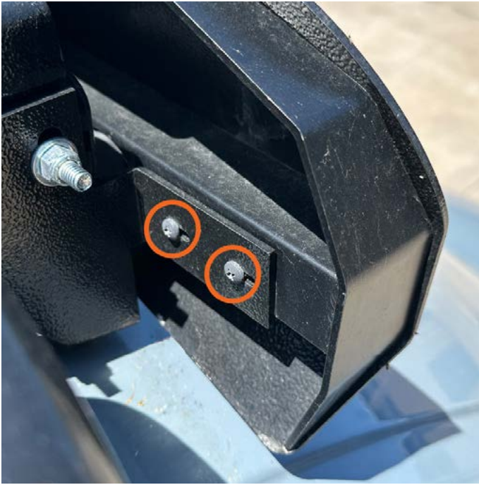
13. Use a Phillips screwdriver to remove the 2 passenger side fairing screws.
