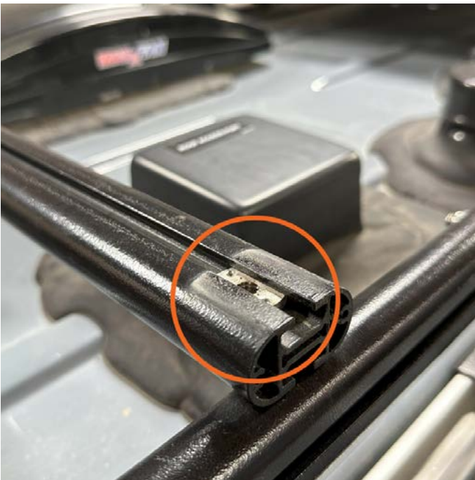
7. Completely remove the bracket and slide out the t-nut.
