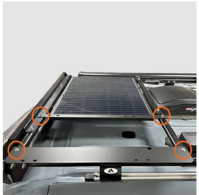
20. Use the supplied \frac{5}{16} "-18x.625" bolts and \frac{5}{16} " washers to install the Agile outer rail onto the 1st and 2nd crossbar brackets. The bolts will go through the crossbar brackets into the t-nuts. Align the Agile inner and outer brackets then fully tighten all nuts and bolts. Torque to 12 ft lbs. Re-connect fairing light connector and zip tie harness to crossbar.
