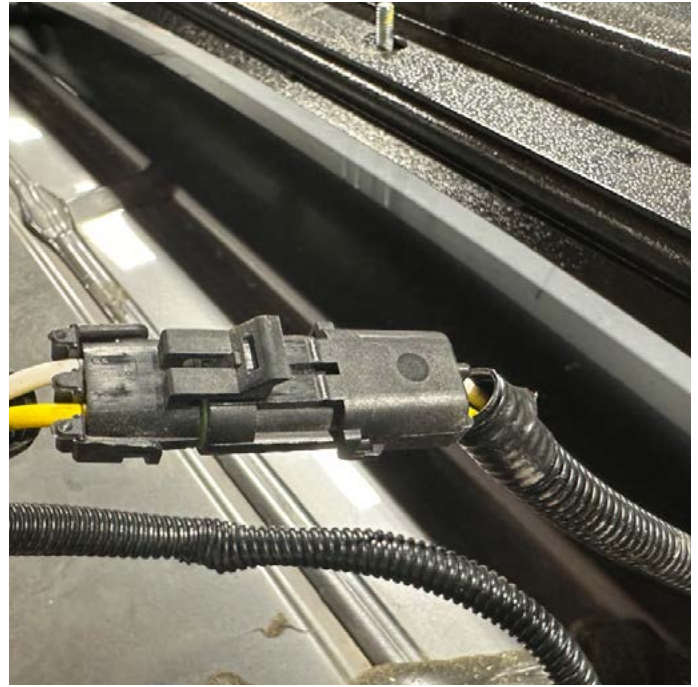
14. Locate the fairing light harness. Cut off zip ties and unplug at connector. With the help of an assistant, lift fairing from cross-rail and remove fairing completely.
