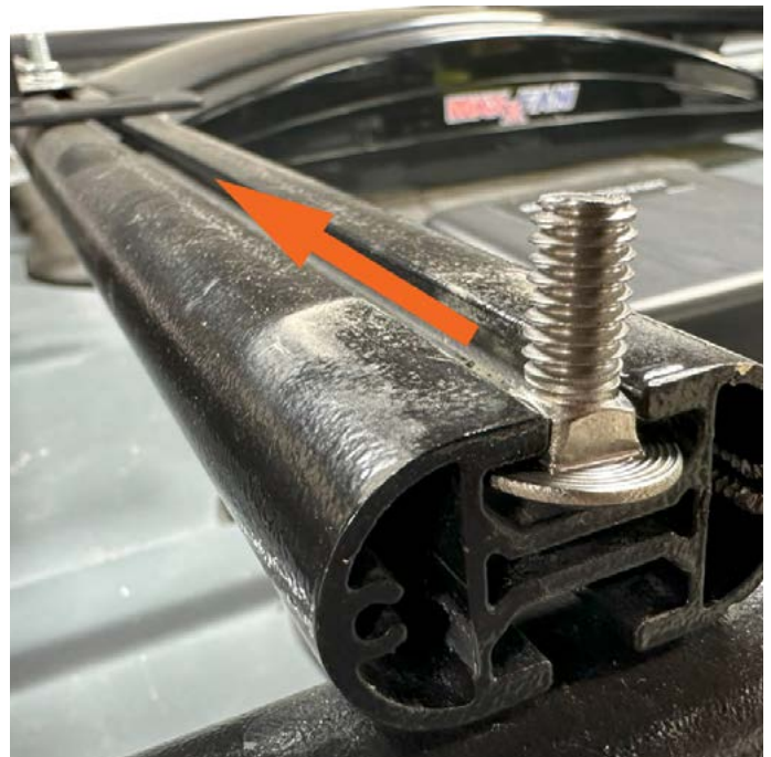
8. Install one of the supplied 5/16"-18x1" carriage bolts into the cross-rail. Slide carriage bolt in towards solar panel.
