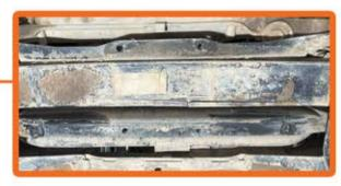
**2.** Use a 13mm wrench/socket to remove the square leaf spring plate.
