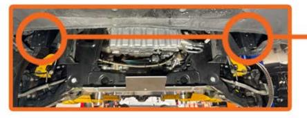
**1.** Use a 13mm wrench/socket to remove the lower radiator support bracket.
