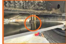
**6B.** Use the two supplied M8x1.25x100mm bolts, 19mm x73mm spacers, and M8x1.25 flange nuts to bolt the Rear Engine Skid Plate to the rear engine crossmember using the factory holes. \*\*Hand Tight Only\*\*
