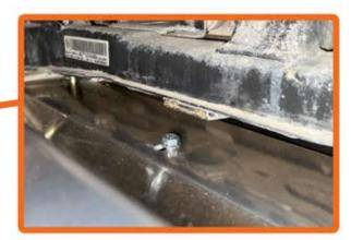
**8B.** Use one of the supplied M8x1.25x25mm bolts and flange nut to bolt the center of the Trans/Tranfer Case Skid Plate to the Rear Engine skid plate.
