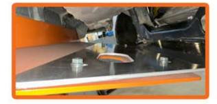
5. Bolt the Front Engine Skid Plate to the Rear Engine Skid Plate using four of the supplied M8x1.25x25mm bolts and M8x1.25 flange nuts.
