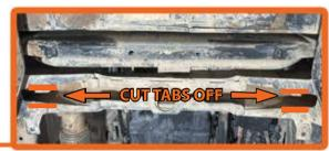
**6.** Use a cut-off wheel or recipricating saw to cut the two tabs of the rear crossmember.
