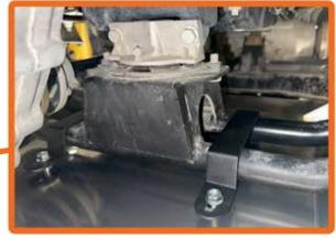
8. Install the Trans/Transfer Case Skid Plate over the Rear Engine Skid Plate. Use four of the supplied M8x1.25x25mm bolts and flange nuts to bolt the plate to the mounting brackets as shown above. \*\* Hand Tight Only\*\*
