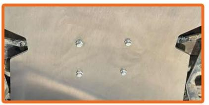
**3.** Install the Rear Engine Skid Plate using four of the supplied M8x1.25 x 25 bolts. The plate will bolt on to the four leaf spring plate holes. \*\*Hand Tight Only\*\*
