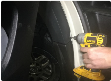
install molding screw
