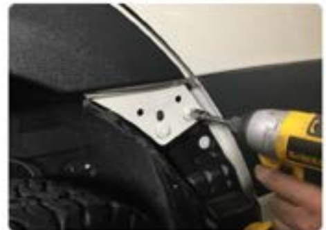
install fender bolts
