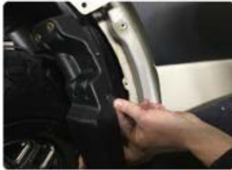
install speed nut
