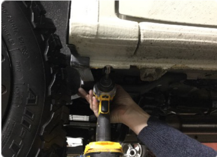
remove lower 10mm nut
