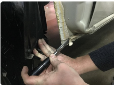
remove excess sealant
