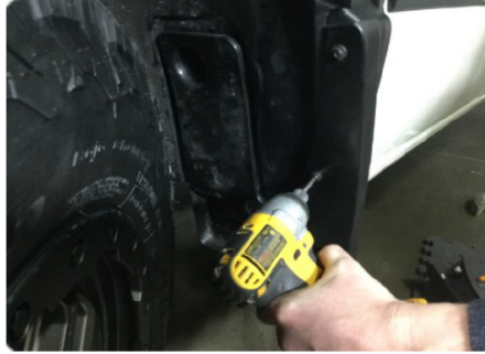
install T-25 screws
