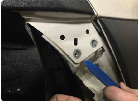
pry fender from sill
