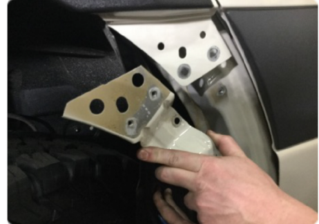
bend sill down and pull
