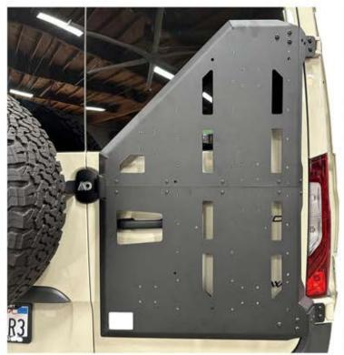
9. The installation of the RDO plate assembly will require two people. One will hold the assembly, while the second person installs the mounting hardware.
