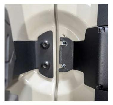
15. Line up the RDO plate assembly center mount with the new emblem bolts.
