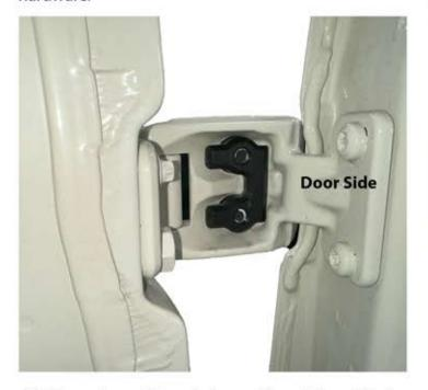
11. The c-shaped threaded mounting plate will index into the two factory hinge holes and will sit in the inside hinge pocket (as shown). Hand tighten bolts.
