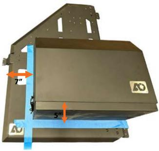
7. To install a box, place your box on the RDO plate assembly. Maintain the minimum clearance (as shown) to avoid clearance and/or parking sensor issues. Use masking tape to mark the final box location. \*\*\* Note: Placing items beyond the right side of RDO plate may block brake light visibilty\*\*\*
