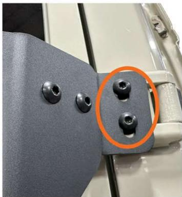
10. Start with the upper hinge. Use (2) of the supplied 3/8-16 x 3/4" bolts and the c-shaped threaded mounting plate. \*\*\*Note: Apply a drop of blue loctite to the bolts\*\*\*
