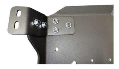
3. Install the upper hinge bracket to the top of the RDO plate assembly (as shown) using (5) of the supplied 3/8-16 x 1" bolts and nyloc nuts. Torque to 31 ft lbs.
