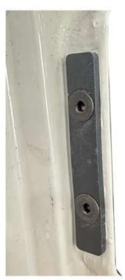
14. Remove factory door emblem. Install the (2) supplied 1/4-20 x 1/2" cap screws and rectangular backing plate into the factory emblem holes.
