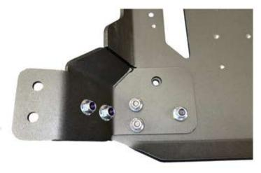
4. Install the lower hinge bracket to the bottom of the RDO plate assembly (as shown) using (5) of the supplied 3/8-16 x 1" bolts and nyloc nuts. Torque to 31 ft lbs.
