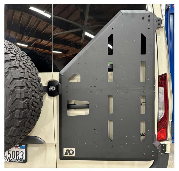
17. Tighten the upper and lower hinge bolts and the two emblem bolts. Torque hinge mounting bolts to 31 ft lbs and the emblem bolts to 8-10 ft lbs. Install your box and/or accessories using (not supplied) 1/4-20 bolts and 1/4" washers.
