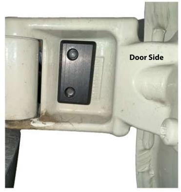
13. The rectangular threaded mounting plate will index into the two factory hinge holes and will sit in the inside hinge pocket (as shown). Hand tighten bolts.
