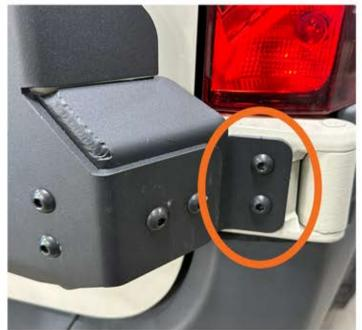
12. Use (2) of the supplied 3/8-16 x 3/4" bolts and the rectangular threaded mounting plate to mount the RDO plate assembly to the lower hinge. \*\*\*Note: Apply a drop of blue loctite to the bolts\*\*\*
