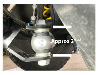
**3.** Use the two supplied 15mm ID thick washers to install the AO/Fox steering stabilizer to the driver side factory location. \*Note: It may be necessary to slightly pry open the oem mount to fit the new stabilizer.\* Apply a small drop of the supplied red loctite to the factory bolt and install using the factory nut.
