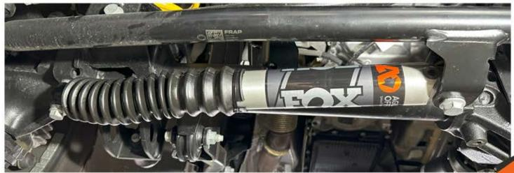
**4.** Torque the passenger side bolt to 75 ft lbs and the driver side bolt and nut to 110 ft lbs. Test cycle the steering lock to lock before driving.
