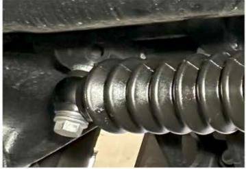
**2.** Use the two supplied conical washers and the 12mm ID thick washer to install the AO/Fox Steering Stabilizer to the passenger side factory location. \*Note the orientation of the conical washers.\* Apply a small drop of the supplied red loctite to the factory bolt and install hand tight.
