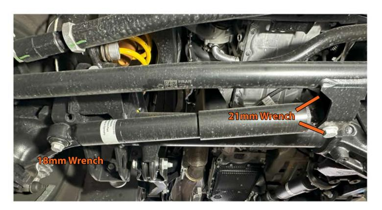
1. The installation of the AO/Fox Steering Stabilizer can be performed with the vehicle on flat ground. Use a 18mm socket/wrench to remove the passenger side bolt. On the driver side, use two 21mm socket/wrenches to remove the nut and bolt. Completely remove the OEM steering stabilizer. The mounting hardware will be re-used.
