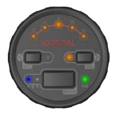
To disable this function hold the valetMode-button until the blue LED lights up. Release the button and the system will return to the normal state.
