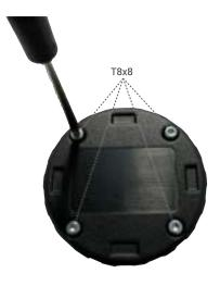
Carefully remove the back cover from the remote. Make sure the printed circuit board doesn't fall out of the housing and remove the battery.
