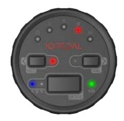
The secure function is still activated for the next power cycle. To deactivate the secure mode press and hold the secureMode-button once more until the blue LED lights up.
