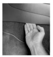
[B, C] The control unit can also be attached to plastic surfaces using the adhesive pads.
