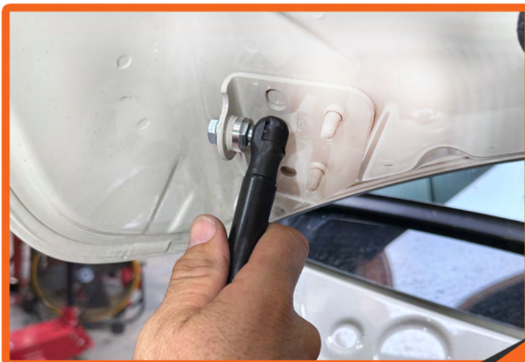
14. Install the hood strut by snapping straight onto ball stud. Strut hole must be centered and straight on ball stud for easy installation.
