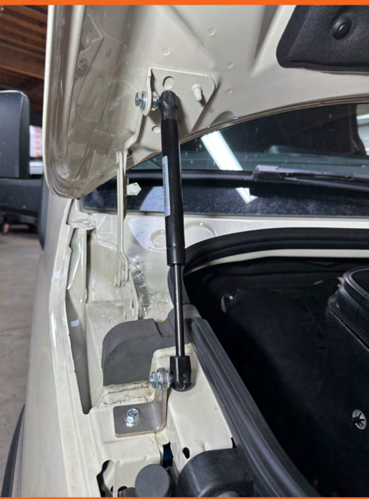
15. Install the hood strut to the lower mount.
