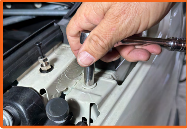
10. Use a 10mm wrench to remove the front upper fender bolt off both driver and passenger sides.
