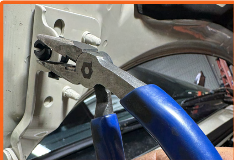
5. Use needle nose pliers to remove the pivot bushing off hood hinge.
