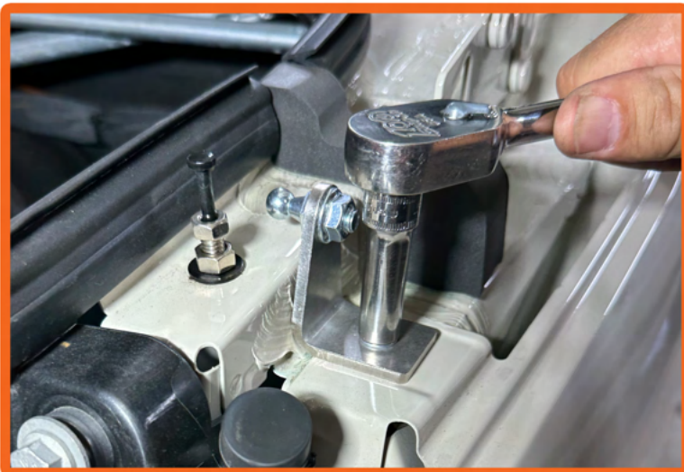
12. Apply a small drop of red loctite to the supplied 6mm-1 flange bolts and install the L-Bracket assemblies.
