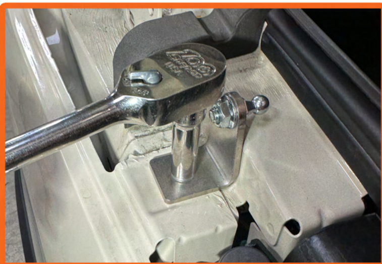
13. Tighten 6mm-1 flange bolts using a 10mm wrench. Torque to 10 ft lbs.
