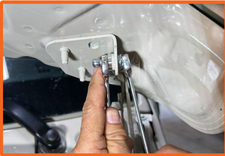
9. Install the second ball assembly on the opposite hinge.
