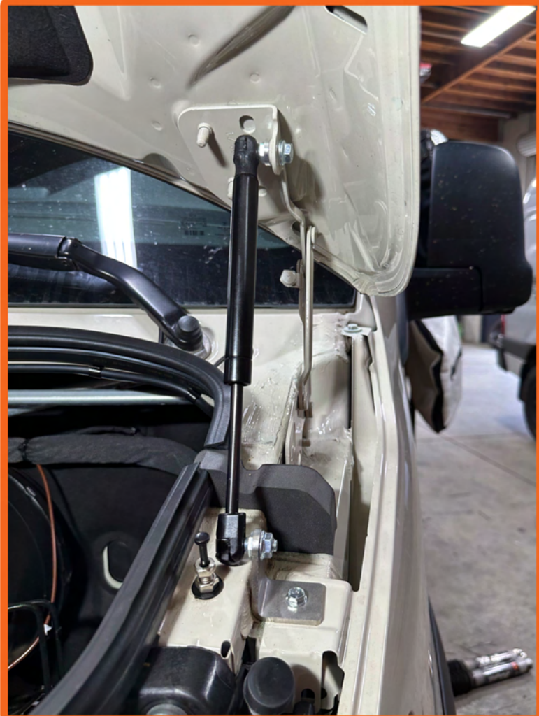
16. Install the hood strut to the opposite side. With both hood struts installed, remove hood prop. Close hood as normal.
