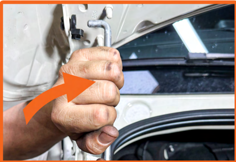
4. Hold the hood support arm with one hand and with the other hand pop the support arm off of the pivot bushing.
