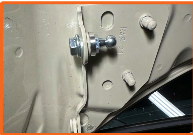
7. Install ball stud assembly onto the hood hinge using the supplied 5/16" flat washer and flange nut.
