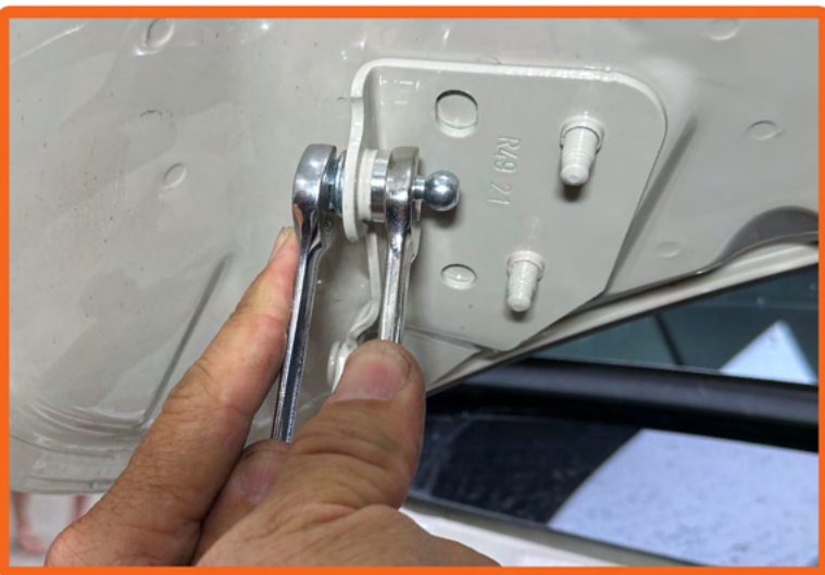
8. Tighten assembly using two 1/2" wrenches.
