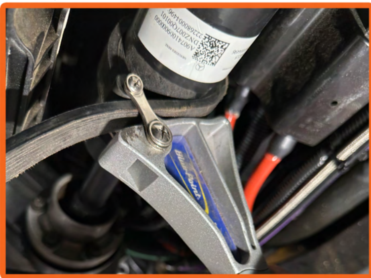
9. If performing work on a lift, use a strap wrench to hold the driveshaft from spinning.
