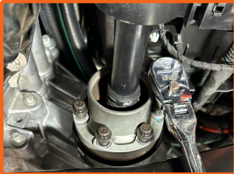
7. Align driveshaft and AO spacer to transfer case flange. Install supplied 12-point bolts with factory 2-hole spacers.
