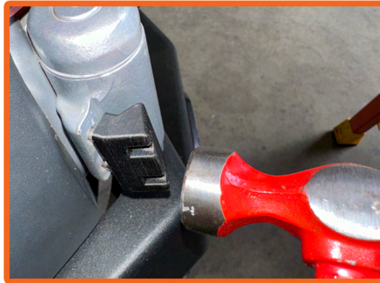
8. Use a hammer and evenly tap the new door stop until flush with hinge. Repeat the same process on both upper and lower hinges.
