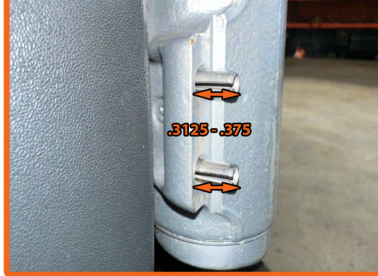
6. Lower Hinge: Roll pins should protrude .3125 to .375 inches.
