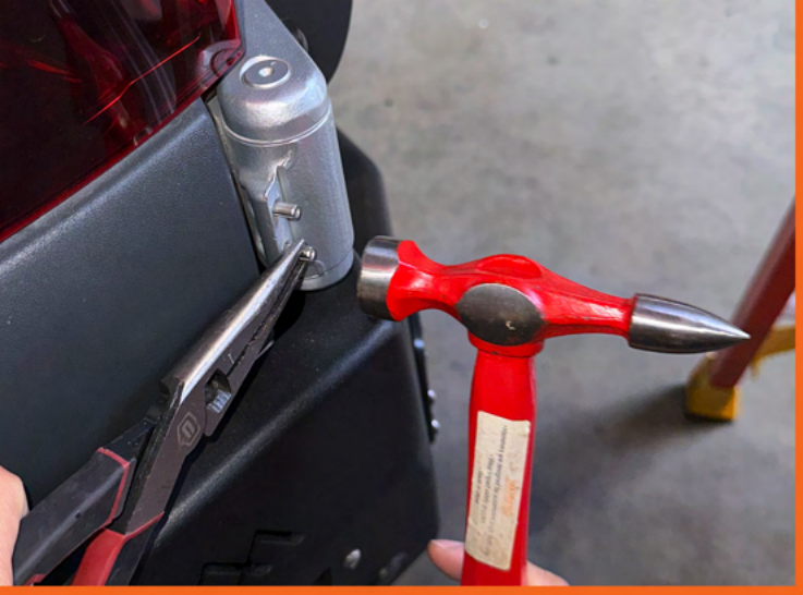
5. Lower Hinge: Hold roll pins with needle nose pliers at hinge holes then drive pins into holes using a hammer.
