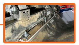
8. Use three of the M8x1.25x30 bolts and three M8x1.25 Flange nuts to install the transmission/transfer case skid plate. Hand tighten only at this time.
