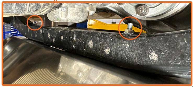
9. Use the two supplied M8x1.25x70 bolts and two flange nuts to install the rear of the transmission/transfer case plate to the tramsmission crossmember. Hand tighten only at this time.
