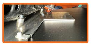
6. Install the front engine skid plate using 7 of the supplied M8x1.25x25 bolts. The front 4 bolts go into the factory override brackets, 2 bolts go into the clip-on barrel nuts, and the center bolt will use one of the supplied M8x1.25 flange nuts. Hand tighten only at this time.
