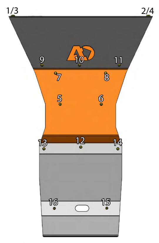
10. Tighten all the bolts following the sequence above. All bolts require a 13mm wrench/socket except for the rear transmission/transfer case plate to transmission crossmember bolts that require a 12mm wrench/socket. Torque all bolts to 23 ft lbs.
