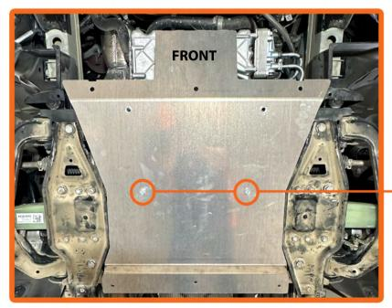
3. Install the mid-section skid plate as shown using the supplied M8x1..25x25 bolts. These bolts will go into the clip-on barrel nuts installed onto the suspension crossmember. Hand tighten only at this time.
