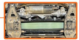
2. Install 2 of the supplied clip-on barrel nuts to the suspension crossmember. Line up the the barrel nuts to the existing holes on the crossmember.
