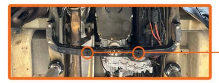
7. Use the existing transmission crossmember holes as guides and drill completely through the crossmember. A 3/8" drill bit is supplied.
