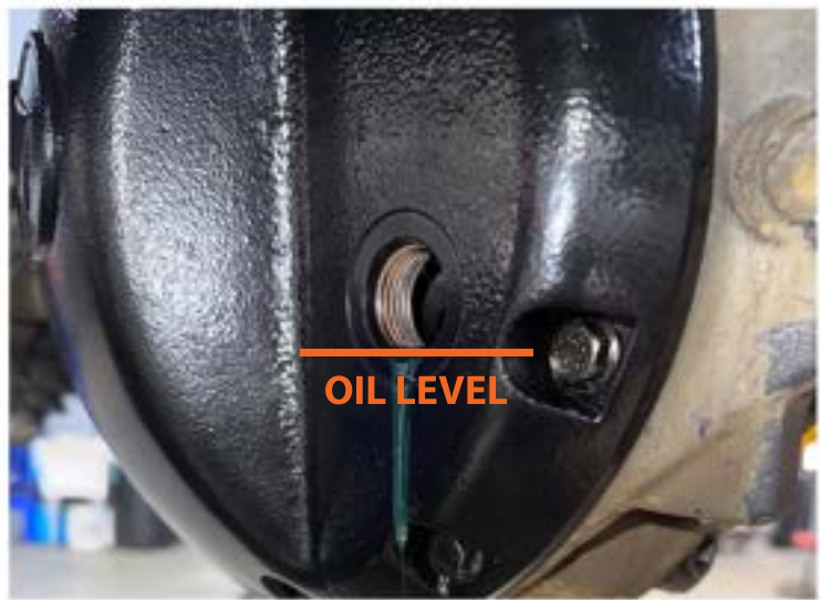
The oil level should be at the bottom of the fill hole.
