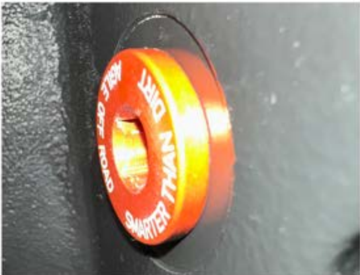
Use a 3/8" drive ratchet to install fill plug. Tighten until fill plug makes contact with AO Diff Cover.
