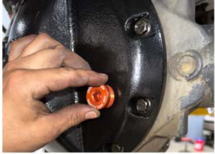
Use a 3/8" drive ratchet to remove the fill plug.
