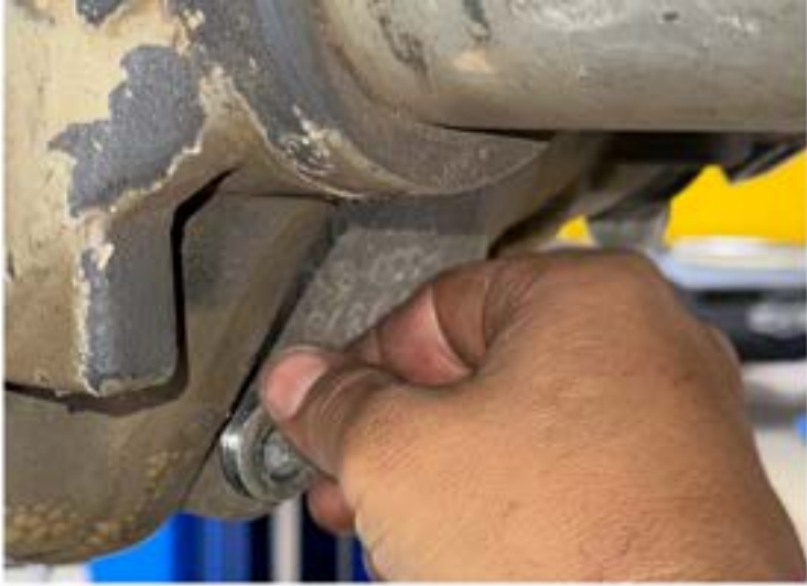
Re-install factory drain plug.
