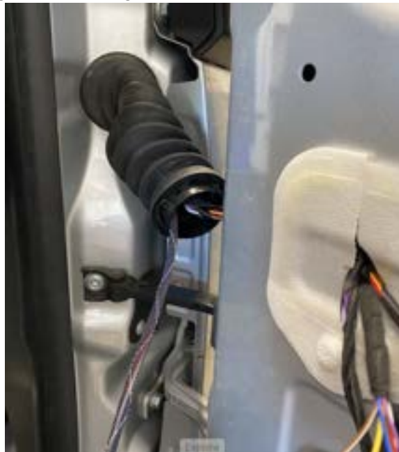
5.7. Run the wires through the inside of the door and out of the opening in the door such that they can be connected to the new speaker.
