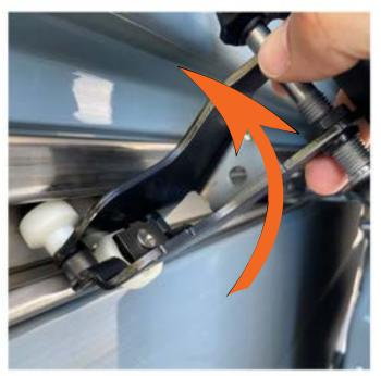
Slide the hinge back away from the sliding door then rotate upwards to remove the hinge from the track.
