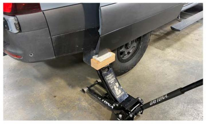
Open the sliding door approx. 3/4 of the way open. Use a floor jack to hold the sliding door up at the original height. Use a block of wood and a rag to protect the door from scratches.
