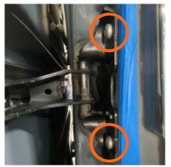
Use masking tape to mark the edge of the original hinge. Use a T47 torx bit to remove the two hinge bolts.
