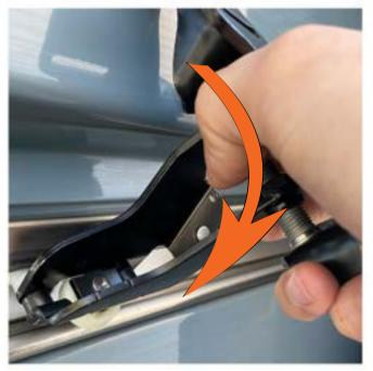
Install the supplied hinge by inserting the upper rollers into the track first then rotating down
