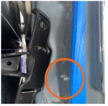
\*Note the two hinge indexing protrusions\*
