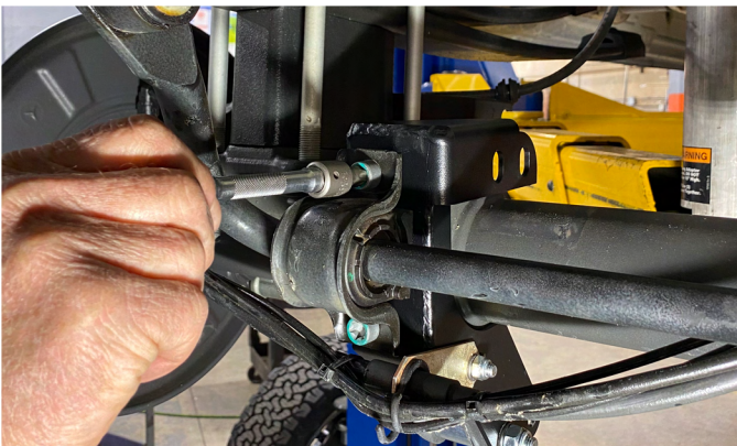
Reinstall sway bar saddle bracket using the factory hardware.
