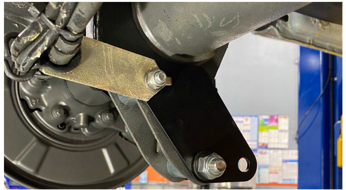
Install the supplied 12mm bolt, sleeve, and hardware to the rear lower bracket holes.
