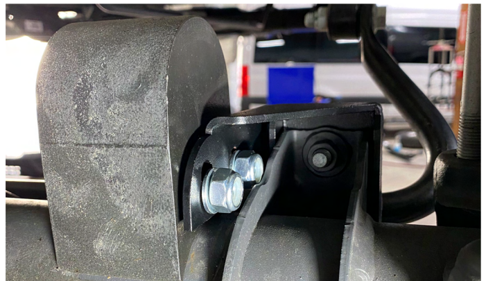
Use the supplied 10mm socket cap bolts, washers, and nyloc nuts to reinstall the factory bump stop extension.
