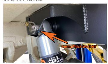
Install rear shocks using the supplied 14mm x 100mm upper bolts . Factory and Fox 2.0 shocks will require the use of the supplied 6mm thick washer. No spacer is required when using Fox 2.5 shocks. Re-use factory lower mounting hardware. \*\*Use red Loctite on bolts\*\*
