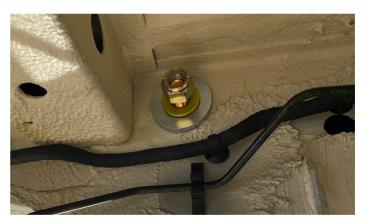
Install the supplied 1/2" large diameter washers, 1/2" small diameter washers, and 1/2" nyloc nuts to the inside of frame. At this time do not fully tighten.
