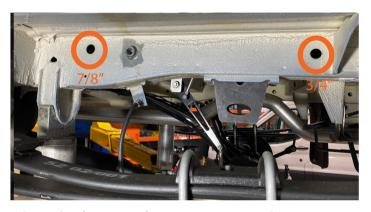
Clean the frame surface as necessary. The 2019+ Sprinter frame comes with two existing holes. The front hole is 7/8" and the rear hole is 3/4".
