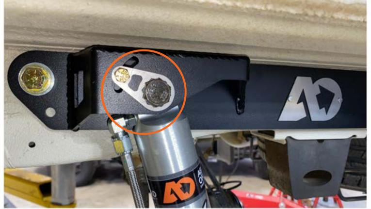
Torque the upper shock bolt to 105 ft lbs then install the bolt locking tab using the supplied 1/4" bolt, washer and nyloc nut. Torque the lower shock bolt to 75 ft lbs. Fully tighten the front and rear AO Shock Mount bolts and torque to 90-100 ft lbs. Repeat same process on the passenger side. Re-install wheels and torque lug nuts/bolts to the recommended wheel torque specs.
