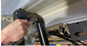
Use a 21mm socket to remove the upper shock bolt. Then use a 18mm socket and wrench to remove the lower shock bolt. Completely remove shock and set aside.
