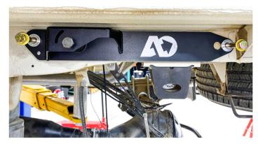
Install the supplied 14mm x 100mm shock bolt to hold the AO Double Shear bracket against frame. Install the 7/8" frame/bolt sleeve through the front hole of the bracket and frame and the 3/4" frame/bolt sleeve through the rear hole of the bracket and frame. Install the supplied 1/2" x 4.5" bolts with washers.
