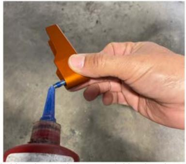
Use an E8 socket and wrench to remove the bolt holding the speed sensor. Apply blue thread lock to the supplied M6 bolt and install the AO Speed Sensor Guard over the speed sensor. Use a 5mm allen wrench and tighten bolt. Repeat on opposite side.
