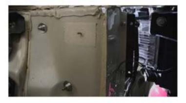
Install the supplied large fender washers and 5/16" nuts from the inside of the wheel well. Have a helper hold the nuts from inside the wheel well while you tighten the bolts from inside the engine compartment.
