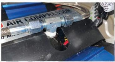
Apply teflon tape to tee fitting threads and install in compressor.
