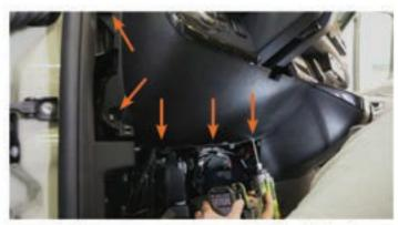
Remove the (5) T-20 torx screws that hold the lower dash panel.
