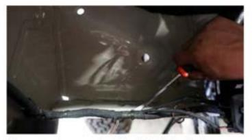
Use a panel removal tool to detach the factory Sprinter harness off of the inner sheet metal panel.
