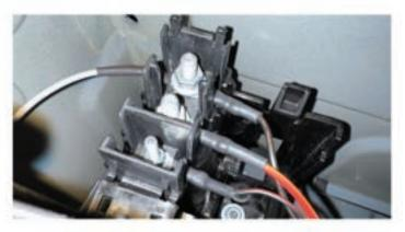
Connect the grey wire ring terminal to the rear terminal stud with the black w/brown stripe wire.
