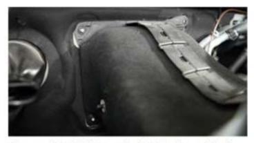
Remove the (4) 10mm nuts holding the cabin air filter box to the firewall and remove air filter box.
