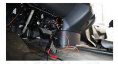
Remove the driver's side plastic cover off of the lower center console. Route the power and switch harness through to the driver side. Use zip ties to fasten harnesses. Re-install tool tray and floor mats.
