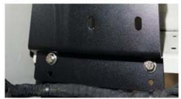
Use the supplied 1/4" hardware to mount the front of the compressor plate to the inner fender sheet using the existing factory harness clip holes.
