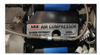
Route the supplied air line from the compressor to the air source brackets. Start with the rear. Be careful to avoid all drive line & exhaust components! Reinstall the air box in the engine bay and any other components you removed during the installation. Test system for operation & leaks. Congratulations, your ARB On-Board Air System installation is complete!
