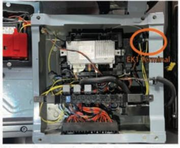
Remove the driver side seat to gain access to the KEY HOT terminal stud (EK1 Terminal). The KEY HOT terminal stud is located in the right rear corner of the seat base. Route the grey key hot from the battery box to the bottom of the of the seat base via the floor tunnel.
