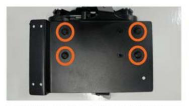
Use the supplied 6mm hardware to bolt the air compressor to the Agile mounting plate.
