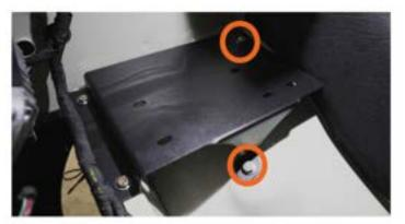
Insert the supplied 5/16" bolts and washers through the compressor plate and inner fender sheet metal using the existing factory holes. \*The compressor plate is pictured above without compressor to show bolt location.
