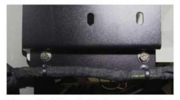
Re-mount the factory Sprinter harness clips to the holes in the compressor plate.
