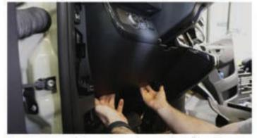
Use zip ties to fasten harnesses and replace battery cover, dash panels, and floor mat.
