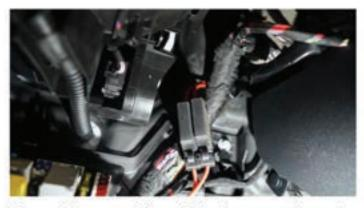
Have a helper carefully pull the harnesses through the boot while you feed them the harnesses from inside the engine bay. Re-install the foam insulation and replace the zip tie.
