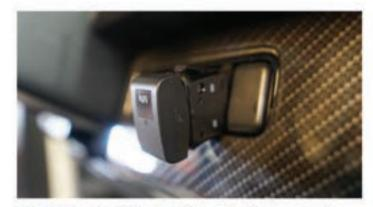
Route the switch harness from the lower console to the switch panel. Install supplied switch onto connector and snap in switch assembly into switch panel. Route the grey wire from the switch connector down towards the the battery box along with the power harness.
