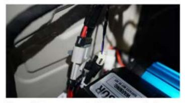
Connect the power and switch harnesses to the ARB compressor.
