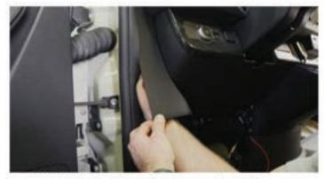
Remove the side lower dash cover by pulling out towards the door. This panel is held on with retainer clips only.
