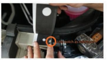
Use the supplied template to mark the air bracket location on the passenger headlight mount.
