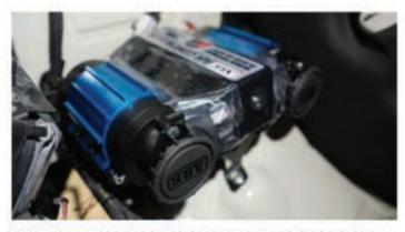
Remove the red factory installed dust plugs and install the air filters.
