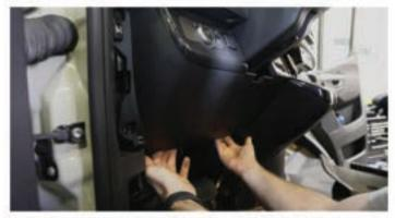
Remove the lower dash cover by pulling on the bottom edge of cover and working around to the outer edges.
