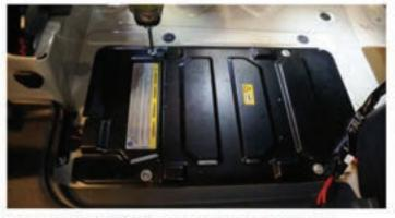
Remove the (2) T-20 torx screws that hold the driver side floor mat edge trim. Remove edge trim and floor mat. Remove the (4) T-30 torx screws that hold the battery cover and remove cover.
