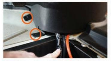
Remove the (2) T-20 screws holding the bottom console plastic to the floor. Route the power harness and the grey key hot wire down to the the battery box. Re-install the (2) T-20 screws.
