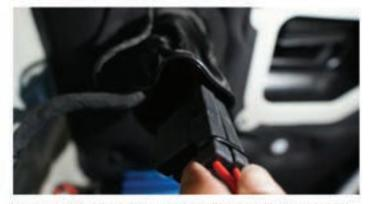
Cut the zip tie off of the firewall pass through boot and remove the foam insulation found inside. Route the compressor power and switch harness through the boot.
