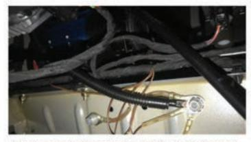
Attach the compressor ground wire to the factory ground stud located below the compressor plate.
