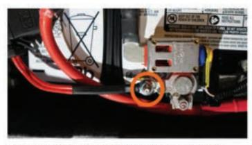
Use the supplied 8mm nut to attach the power harness terminal ring to the positive battery stud.
