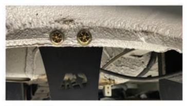
Drill 2 holes & mount rear air source bracket on the pinch weld near the rear bumper. Any location along the rear will work, but we recommend installing it on the opposite side of the exhaust.
