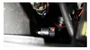
Power off vehicle and disconnect the battery at the battery ground terminal located on the firewall behind the center console.
