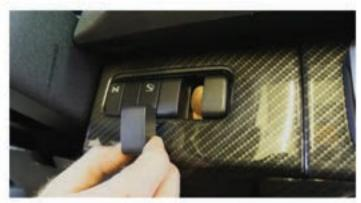
Remove one of the available switch blank covers. To remove cover, reach behind the dash and squeeze the upper and lower tabs of cover while pushing out.
