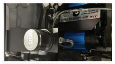
Drill a 5/16" hole at marked location. Line up the notch in the bracket with the notch on the headlight mount. Use supplied hardware to mount bracket.
