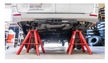
Lift vehicle and support vehicle with jack stands using factory jack points. Remove the rear wheels.
