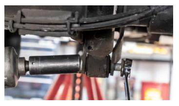
Remove old shocks starting with the lower bolt. Discard the shocks. Save factory hardware, you'll reuse it.
