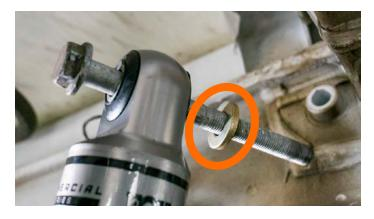
Clean the factory hardware. The included washers are to be installed between the shock body & the frame rail.
