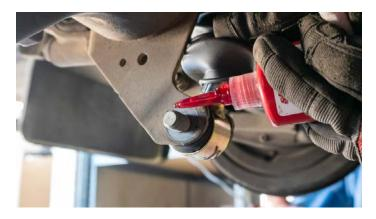
Apply thread-locker and install the lower shock hardware.
