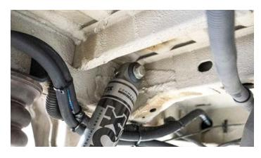
Install new shocks (boot-side down) and shock bolts on the inside of the frame rail.
