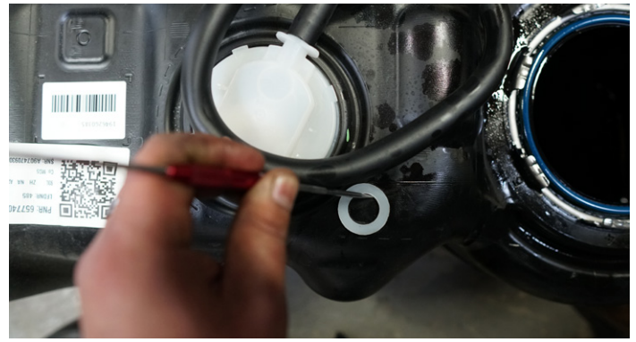
Find the flat spot on the lower right side of the tank ventilator. Use an included nylon washer as a template to mark where you'll drill into the tank to install the RETURN line.
