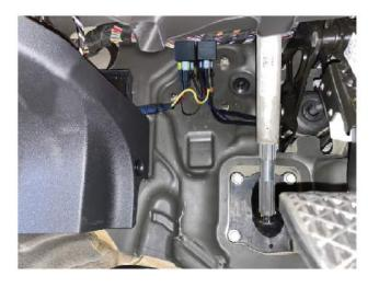
Start light harness installation from inside the van. Mount relays as shown and route switch connector to switch bezel. Route grey wire (pins #4 & #7) to keyed 12v power source.
