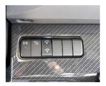
Remove the Torx screws along the bottom & side of the dash to access the back of the blank factory switches. Pop out a switch blank. Install the new switch into the dash.
