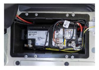
Access the main battery in the driver side foot well. Install the main power wire on the positive battery terminal post using the supplied fuse holder.
