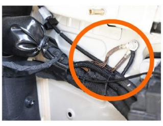
Cut the zip-tie around the boot of the firewall cable pass-through on the driver side. Remove the foam insert inside. Pass the ground and light wires through it. Ground to the factory stud inside the hood. Reinstall the foam insert. Zip-tie the boot closed. Connect the plugs for the lights and secure the wires with zip-ties.
