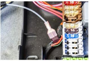
Remove the floor mat and access the fuse box located under the front passenger seat foot well. Connect the grey wire to a KEY HOT power source, using the included wire tap.
