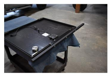
If your Revel is equipped with a smaller 100-watt front panel install the square crossbar so that the panel is offset towards the passenger side when installed on the vehicle. This it to keep the satellite antenna uncovered for optimal reception.
