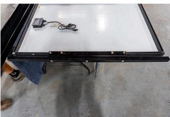
Remove the (2) brackets on the rear facing edge of the front panel. Attach (1) included solar panel bracket to the panel using existing t-nuts with screws & washers from the hardware kit. Center the bracket on the panel before tightening everything. Install the square cross bar. Install the hardware into the ends of the square crossbar to make it easier to reinstall the solar panel later. Set this panel aside.
