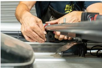
Start by loosening the crossbars and the mounts for any existing roof rack accessories.
