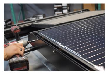
Install the new panel in the middle. Install one side at a time. Use the exposed hardware to keep the panel in place while you work on the other side.
