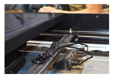
Plug in the middle panel and secure the wire to the crossbar with zip-ties.
