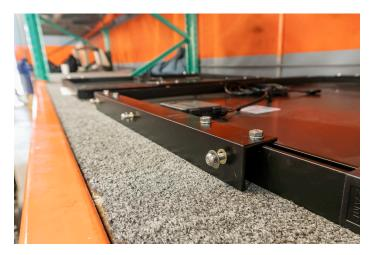
Install (4) included Zamp t-nuts onto each of the shorter sides of the panel included with this kit. Install a solar panel bracket on both short edges of the panel. Center the brackets on the panel (approximately 3.25" from the edge) and tighten. Install the solar panel mounting hardware into the brackets. Set this panel aside.
