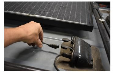
Remove the front panel. Unplug it and take it off of the rack. Take this time to clean the panels & roof if necessary.
