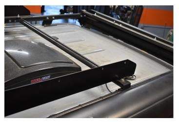
Install the left & right solar panel roof rails onto the Revel roof rack using the existing hardware. The angle cut edge faces forward. Do not tighten the roof rail hardware yet.
