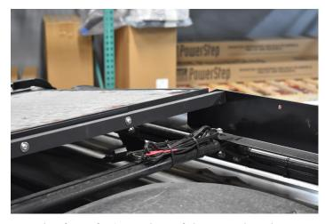
Install the front panel. Start by tightening the hardware on the front facing edge of the panel to the factory roof rack crossbar using the original hardware. Use the included hardware to bolt the square crossbar to the new solar panel roof rails.
