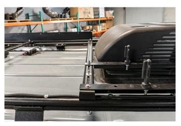
The first two panels dictate the alignment of the kit on your roof rack. With the first two panels installed you may now tighten the crossbars and roof rail hardware.
