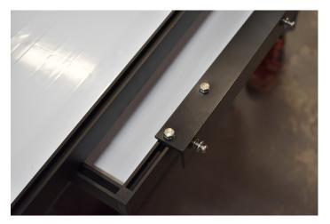
Remove the rear panel from the vehicle. Use a pick to remove the t-nuts from the long sides of the panel. Install (4) t-nuts onto each of the short sides of the panel. Install new solar panel brackets on both short edges of this panel. Center the brackets on the panel (approximately 3.25" from the edge) and tighten. Install the solar panel mounting hardware into the brackets. Set this panel aside.
